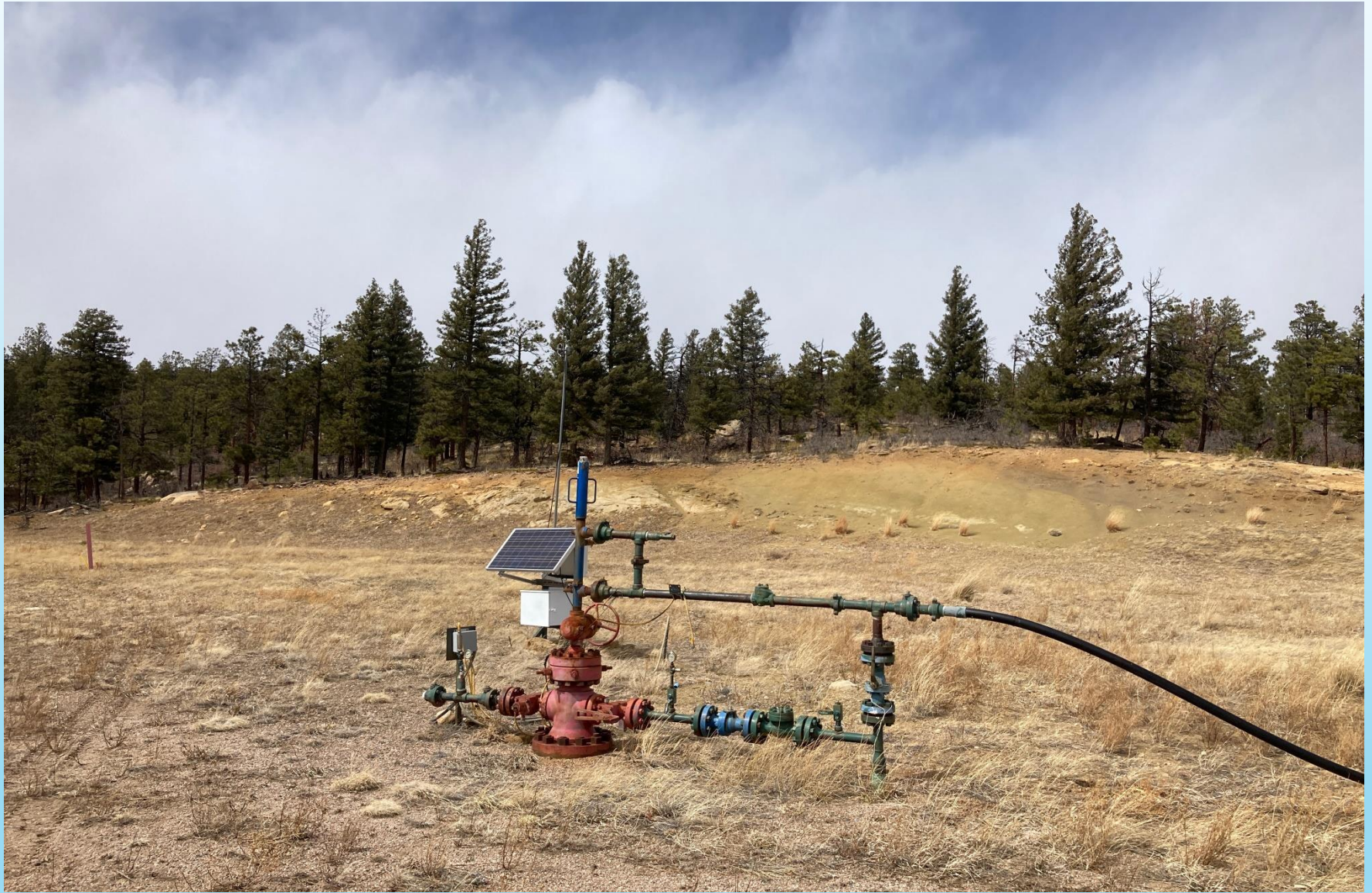
PHOTO 3: WELLHEAD AND EQUIPMENT
