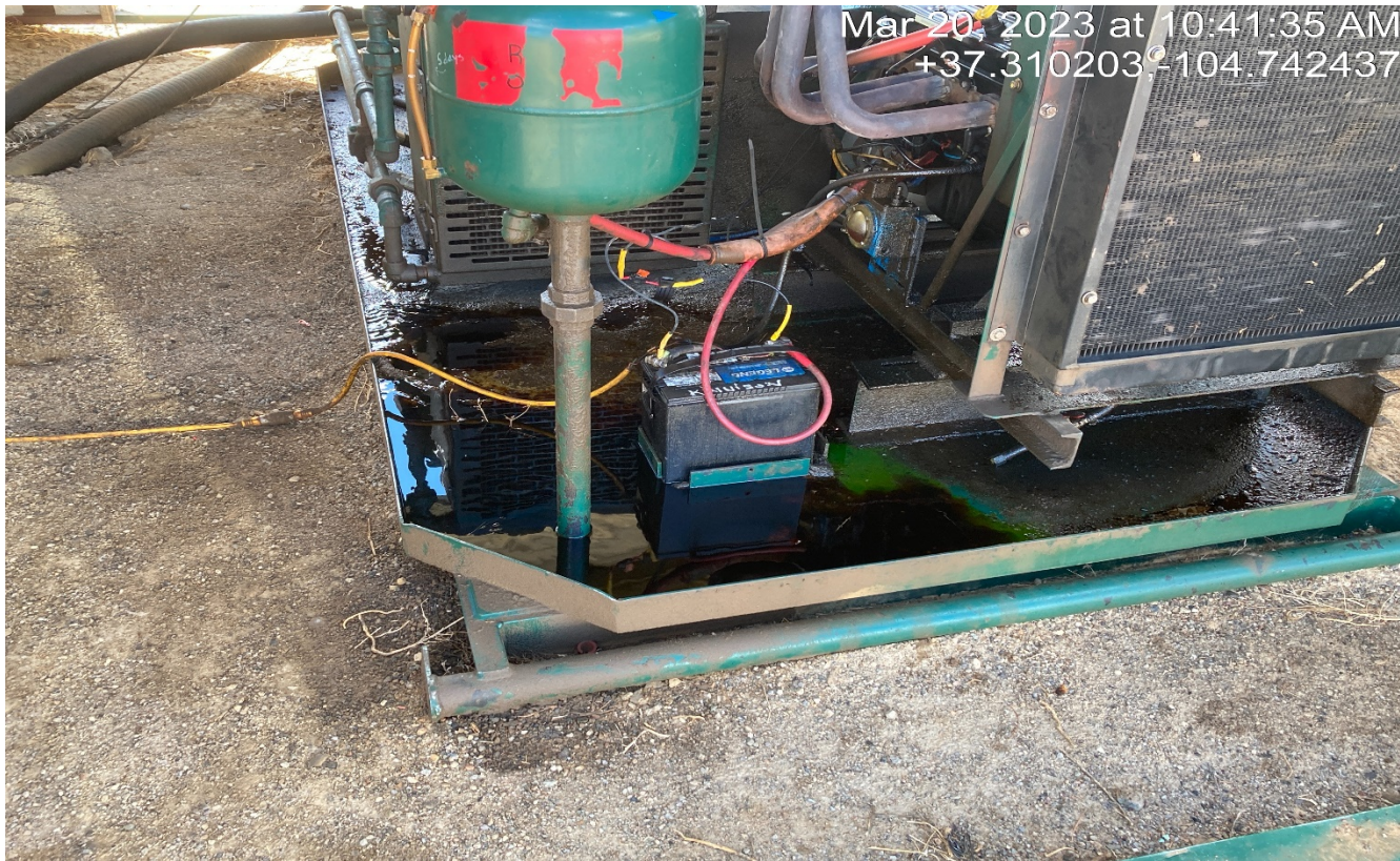
Photo 4. There is oil in the engine skid that needs to be cleaned up.
