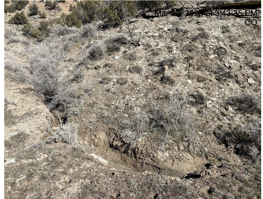
Photo # 2562 Insufficient runoff controls/BMP's – Channel erosion (below berm off SW corner of location)
