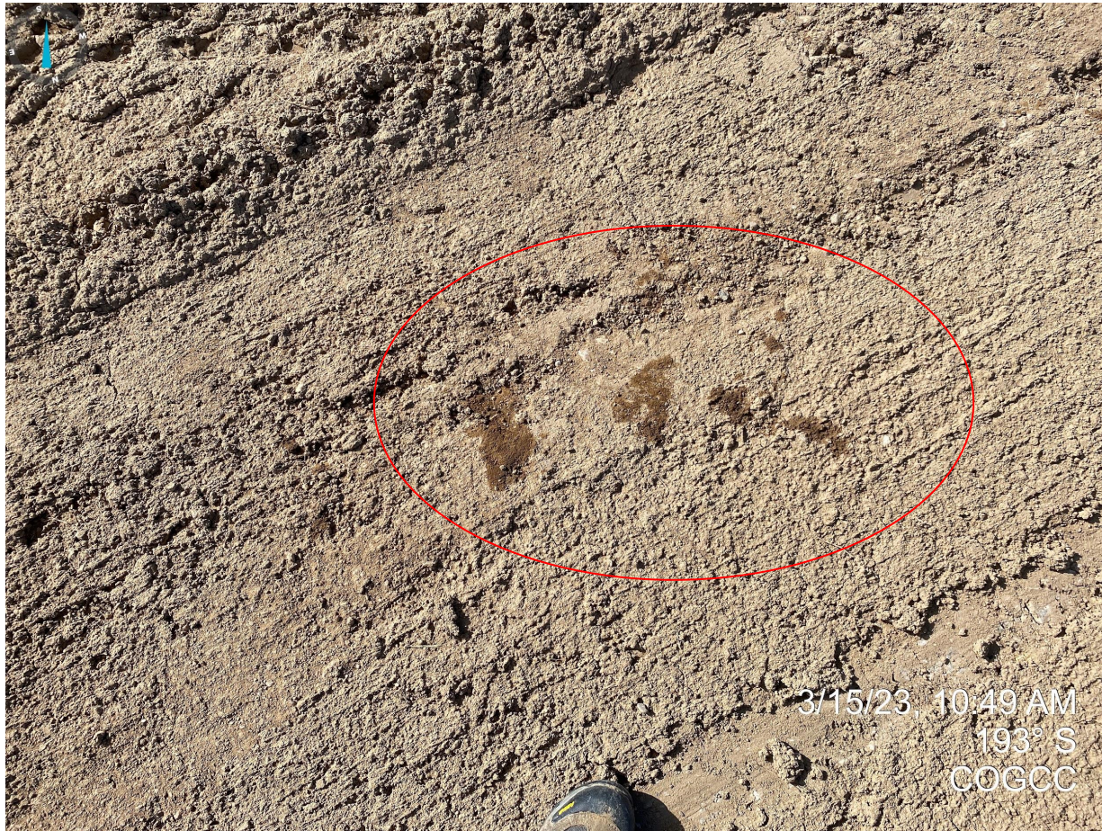
Photo 3. Close up photo of oil stained soil that was near the stockpile material mentioned in Photo 2. This stained soil will need to be properly cleaned up and disposed of per Rule 905.e.
