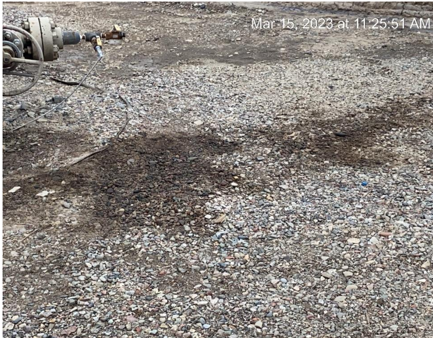
Stained soils around wellhead
