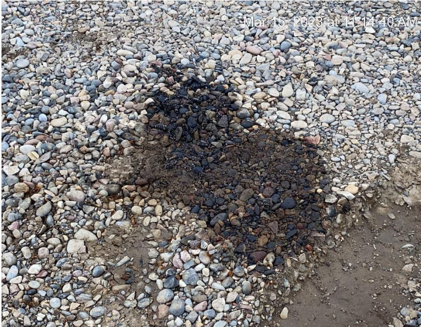
Stained soil at separator
