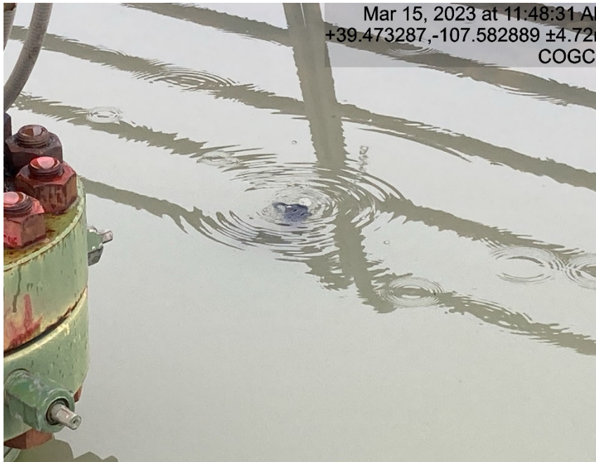
Braden head line leaking
