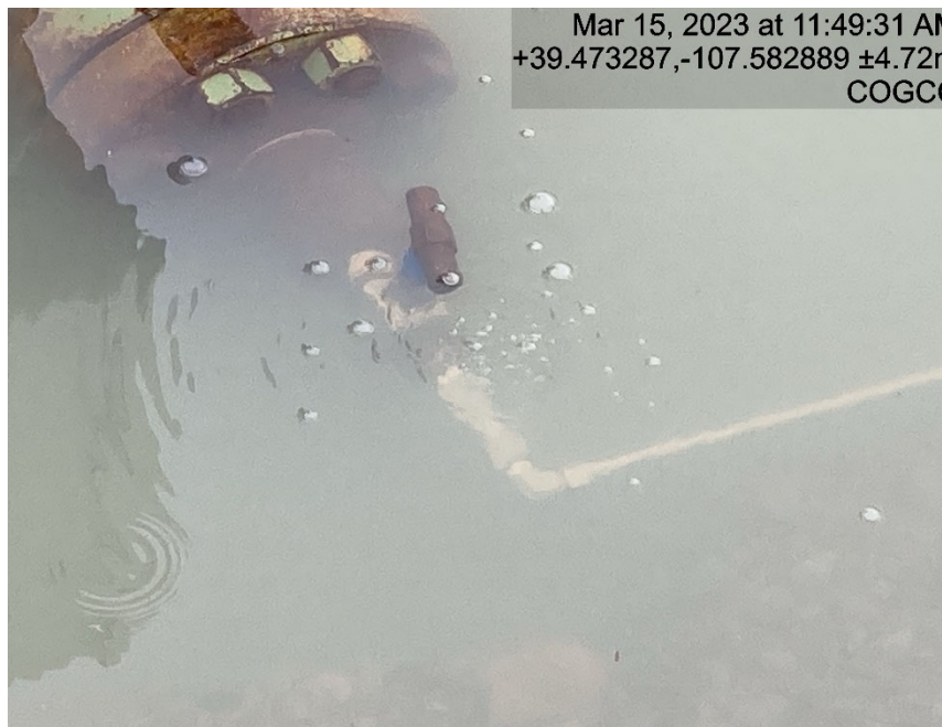
Chemical line leaking
