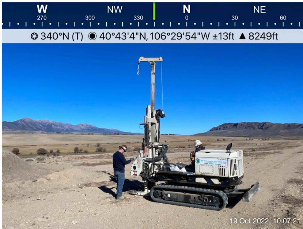
Photo 2: Geoprobe drill rig, 10/19/2022.
