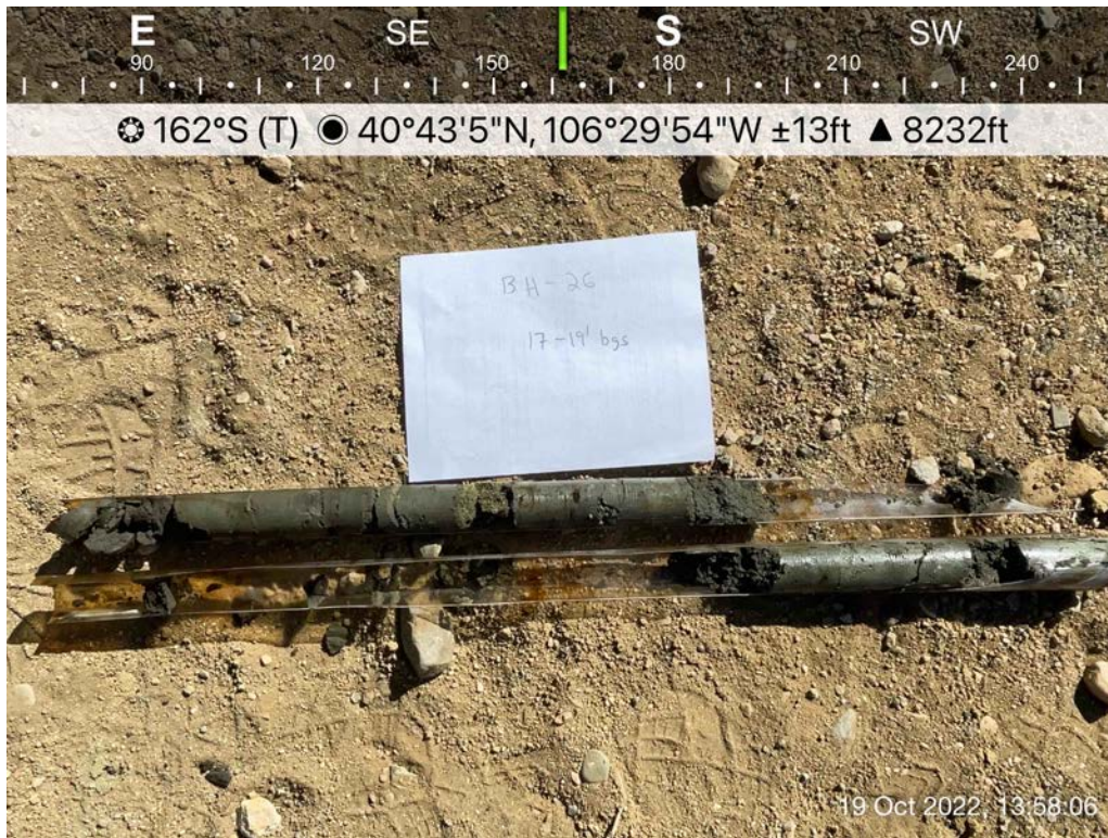
Photo 3: Margaret Spaulding Centralized Tank Battery borehole 26 in Geoprobe sleeve. Oil observed in soil, 10/19/2022.
