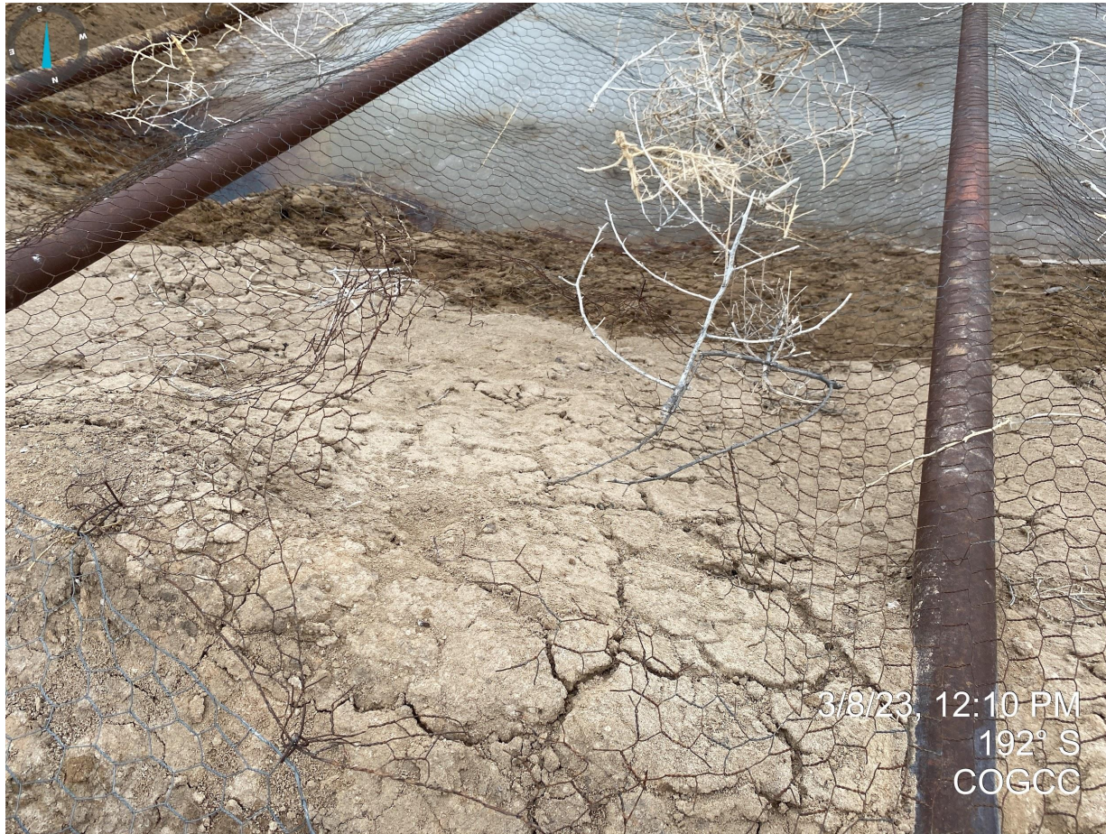
Photo 2. Facing south at pit. Netting is inadequate with large opening observed.
