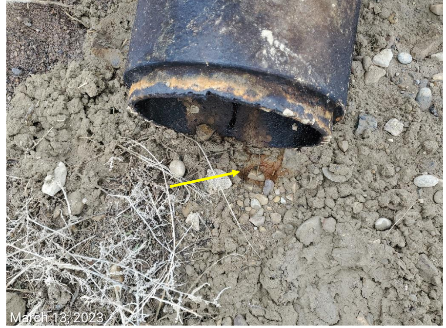
Photo 13: Continued from photo 12. Photo shows what appears to be produced fluids within the disassembled well equipment dripping onto the soil surface.
