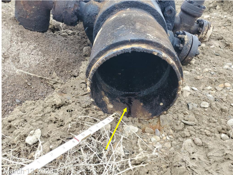
Photo 13: Continued from photo 12. Photo shows what appears to be produced fluids within the disassembled well equipment dripping onto the soil surface.
