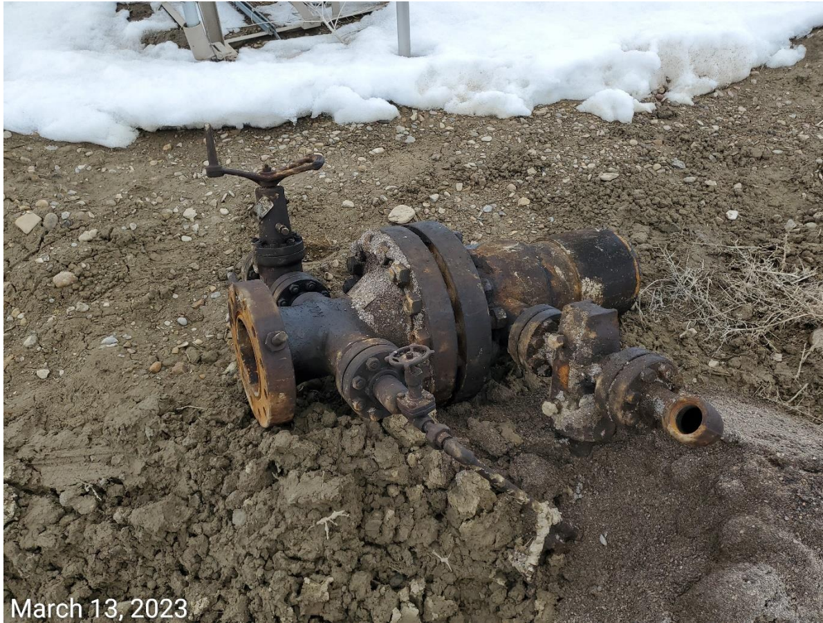
Photo 12: Photo taken from the east end of the Location. Photo shows disassembles well equipment improperly stored on the perimeter of the pad; equipment appears to be covered in production fluids; fluids evident within equipment and observed dripping onto the soil surface.
