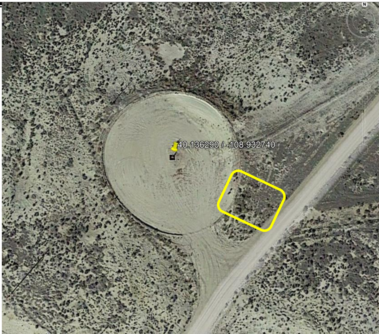
Photo 22: Photo shows a Google Earth Aerial image of the Location. Areas outlined by the yellow polygon represents areas of new disturbance (see photos 20-21). Areas appear to be previously undisturbed, and outside of the designated working pad and access road.
