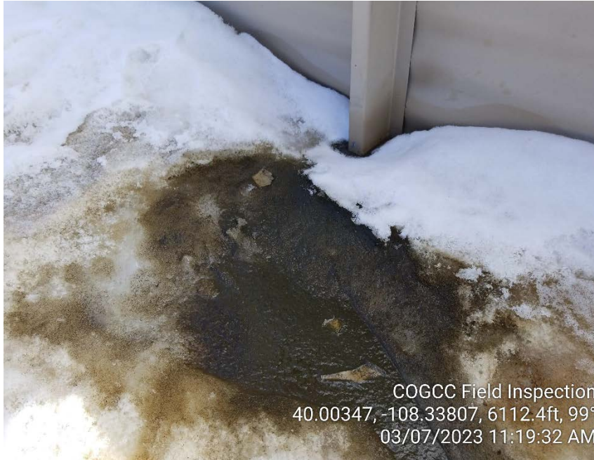
Photo #5 - Localized accumulation of oily waste (hydrocarbon-impacted snow and soil) outside of tank battery and filter pot secondary containment on north side (2).
