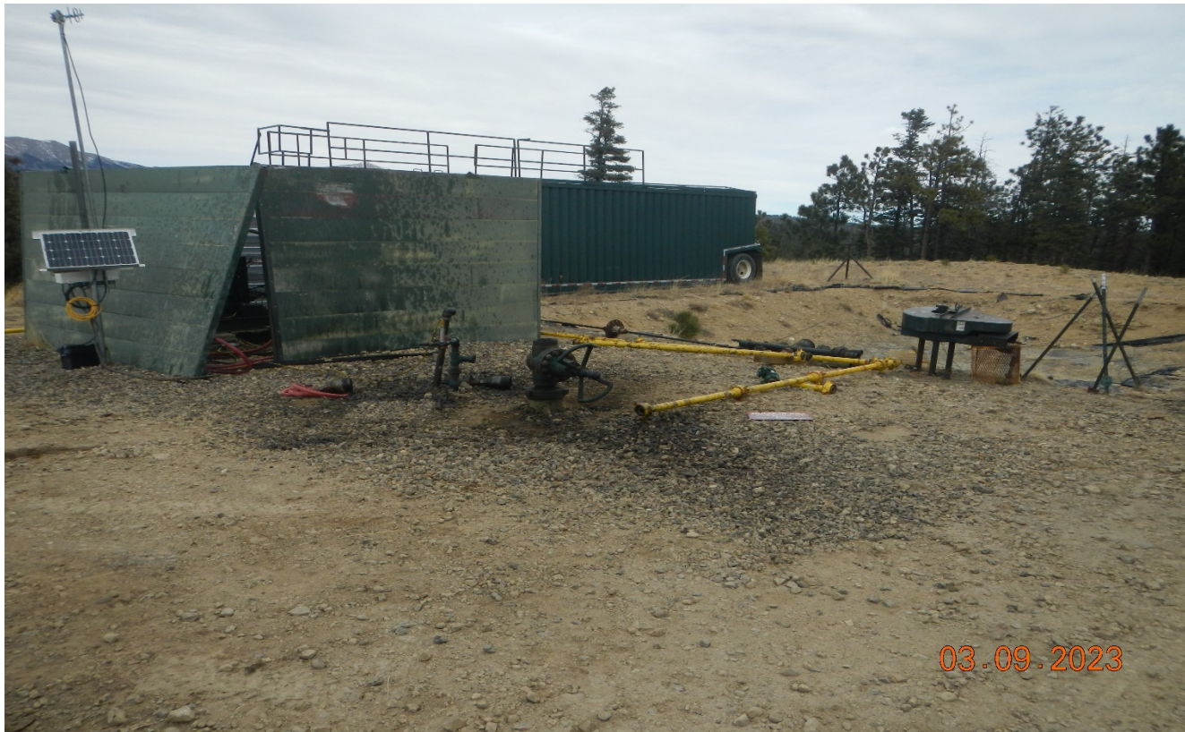
Photo 3. There is oily fluid sprayed out at the onto the ground and engine panels.
