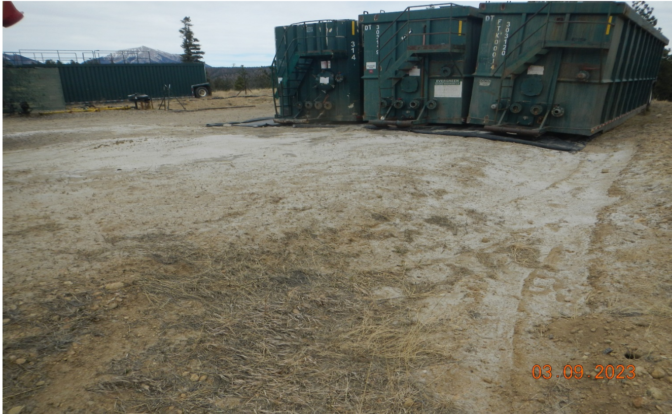
Photo 5. There is frac sand spilled out over the ground that was not properly handled.
