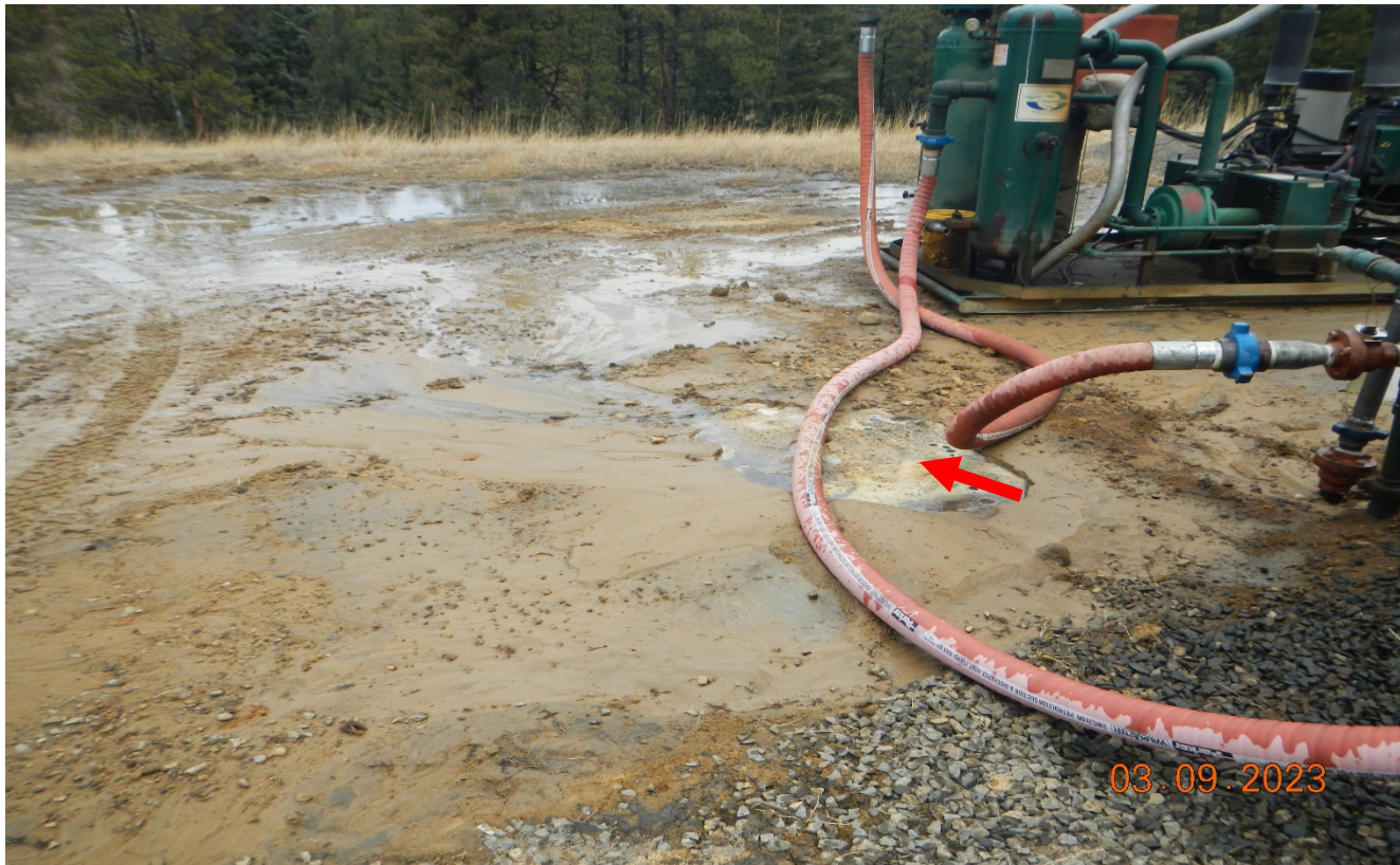
Photo 2. There is a produced water leak bubbling up near the wellhead at the red arrow.
