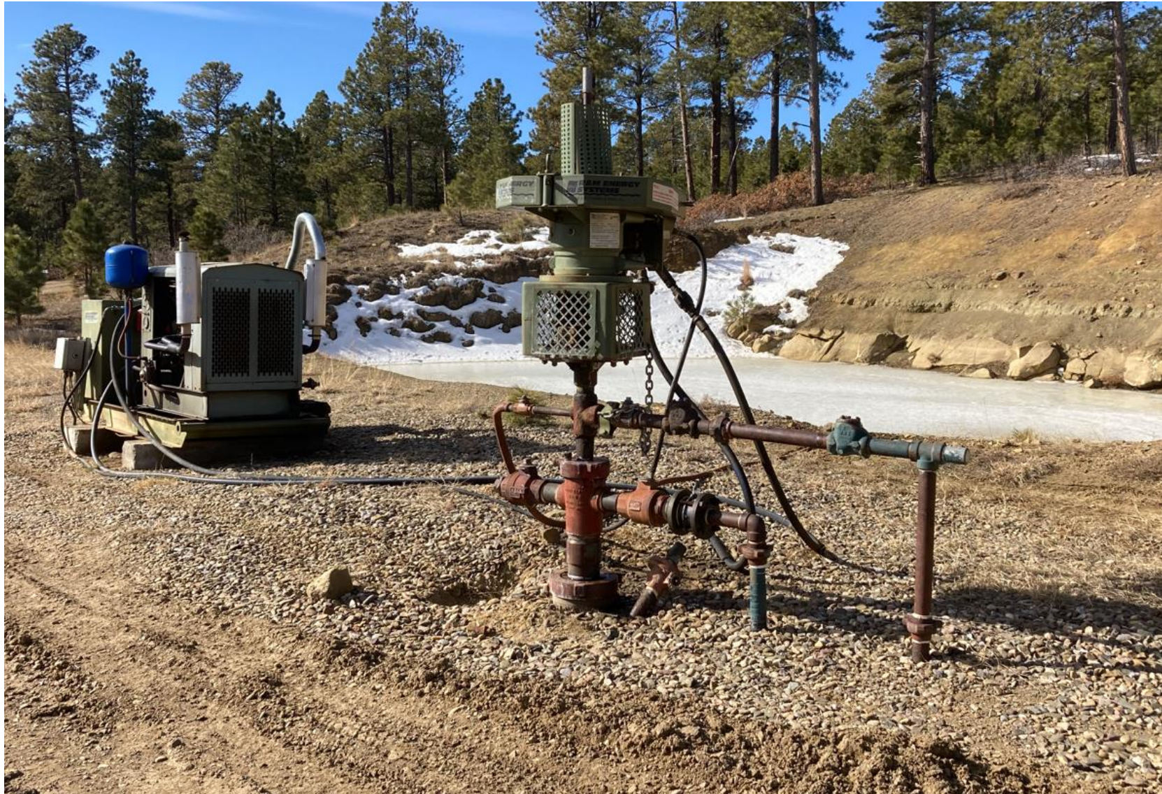
PHOTO 1: THE LEAK AT THE WELL HEAD HAS BEEN REPAIRED AND CLEANED UP TO COMPLY WITH RULE 912.A. ALL VALVES, PIPES, AND FITTINGS HAVE BEEN SECURELY FASTENED AND ALL EQUIPMENT HAS BEEN INSPECTED TO ENSURE GOOD MECHANICAL CONDITION.
