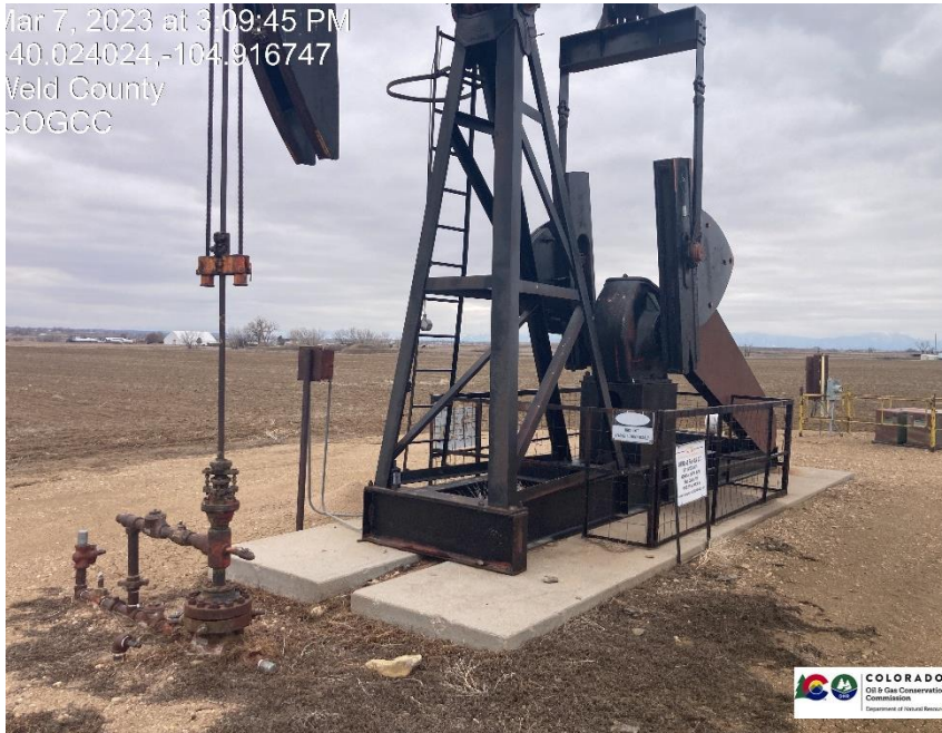
Pic 1 wellhead, pump jack, electric equipment
