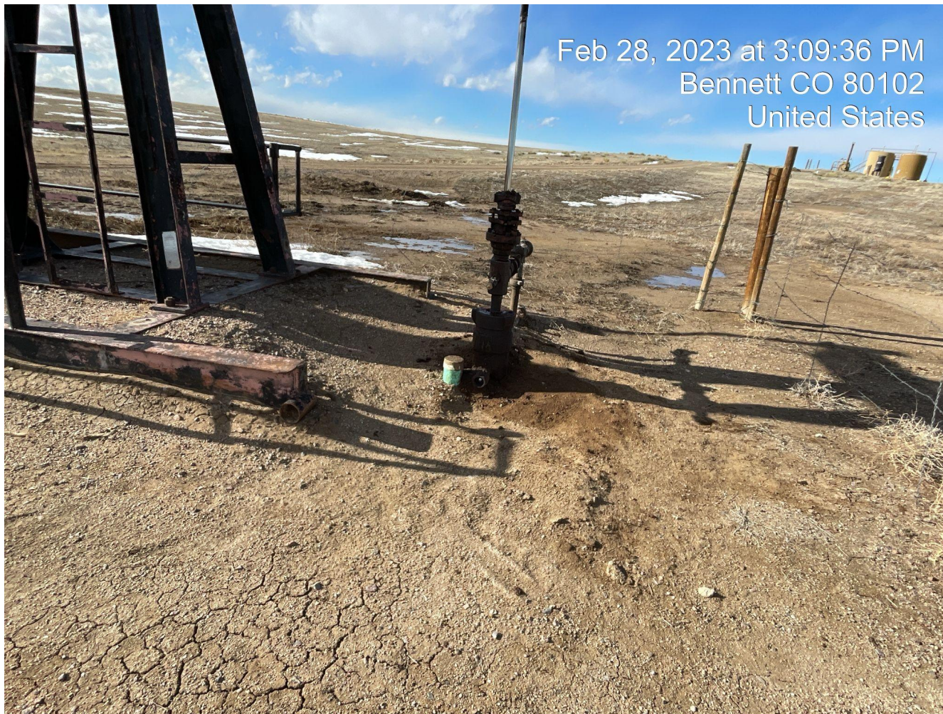
Photo 4. Photo taken of soil staining around well head. .
