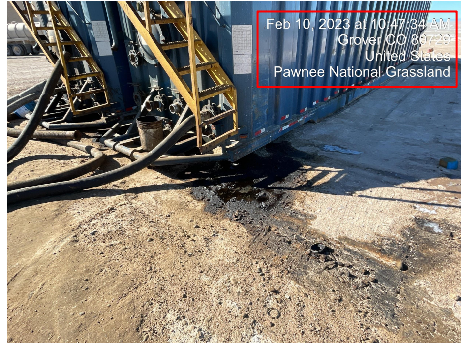
Photo 4. Photo taken from a frac tank on location back on 2/10/23. Photo illustrates frac tank is leaking oily waste. Oily waste appears to be underneath the frac tank.
