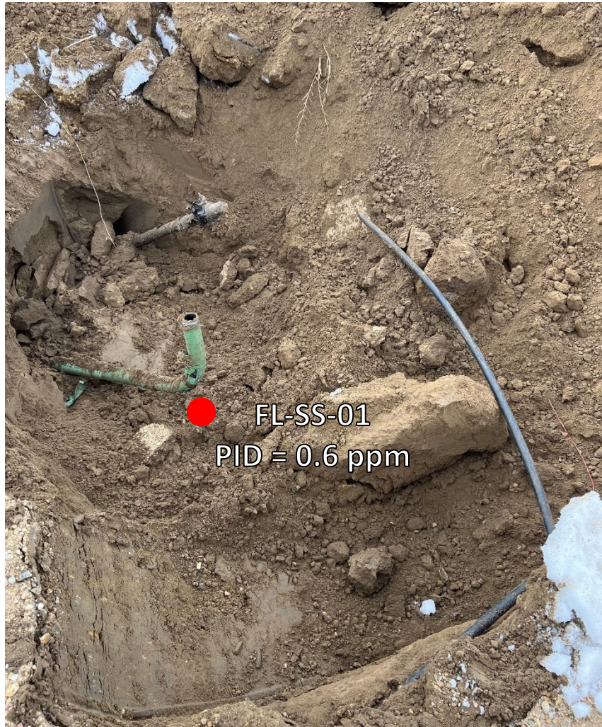
Flowline Terminus/Pt. B at separator – submitted for laboratory analysis
