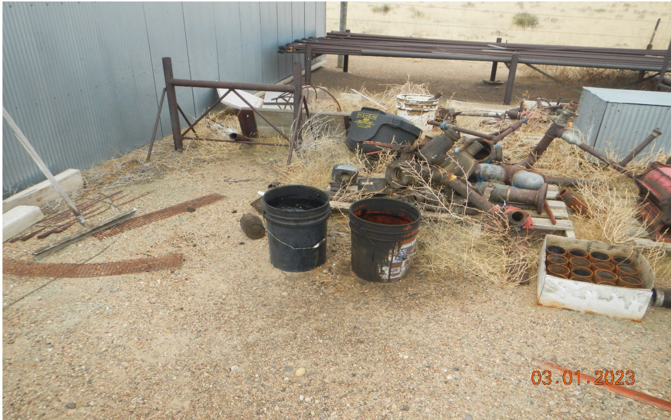
Photo 14. There are various parts and supplies and tow buckets of oil which appear to have spilled out on the ground. Buckets of oil need to be properly disposed and stained soil cleaned up.
