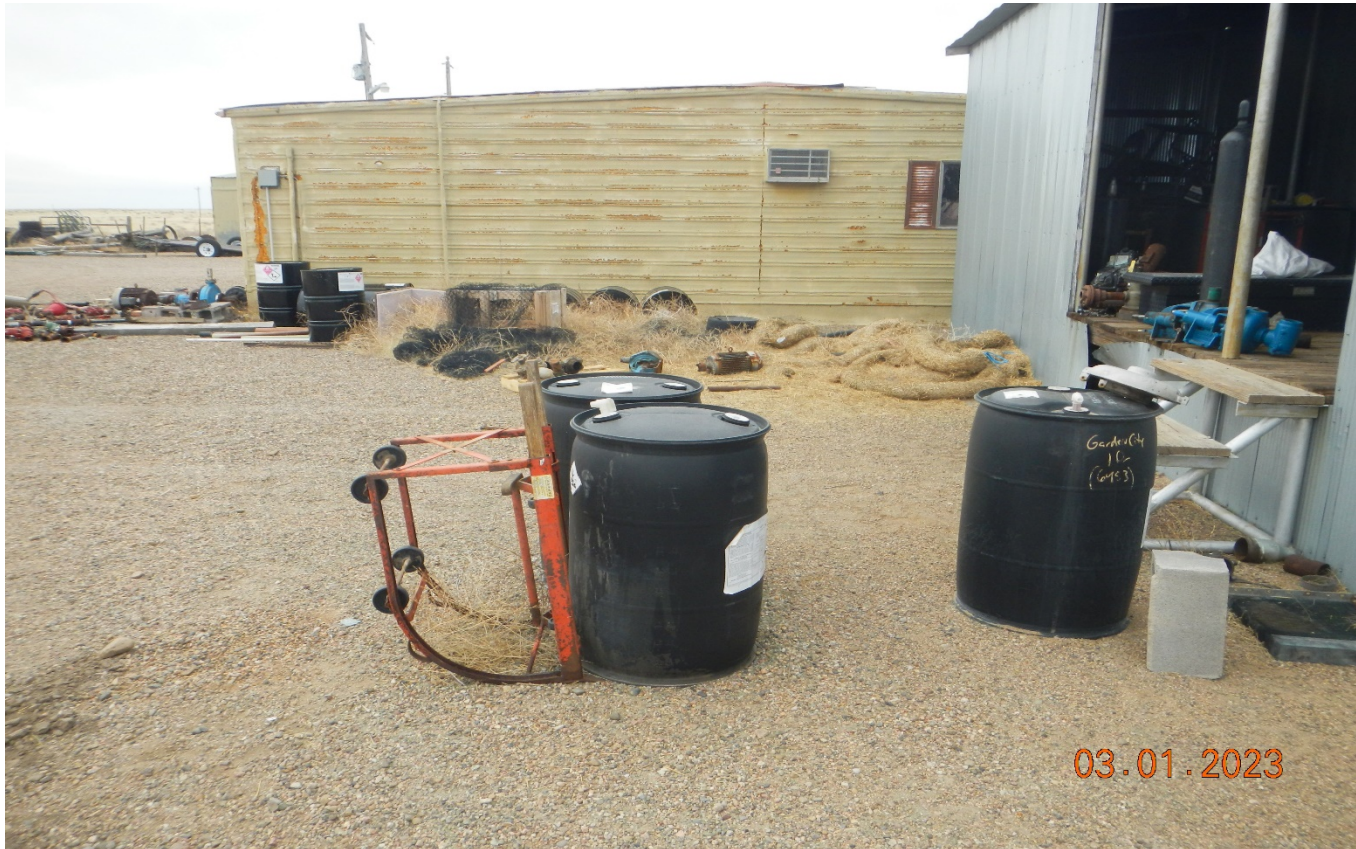
Photo 13. There are several chemical barrals on location with faded labeling and no secondary containment.
