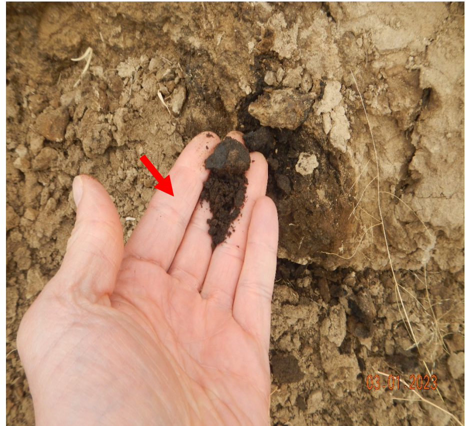
Photo 10. Located at the western side of the spill area. There is an excavated hole at this area approximately 12'x12'6'. There are still areas of oil stained soils at the surface (Bottom left) and 2ft. Down into the excavation area (right photo). Further excavation is needed.
