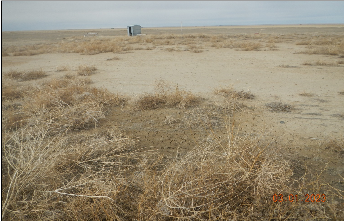
Photo 5. South side of the location facing north. This area approx. 75'x75' is bare of vegetation with no crop growth. There is reason to believe a historic spill has caused impacted soils.
