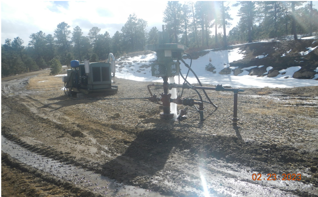
Photo 2. There is ice buildup at the wellhead indication a dripping leak.
