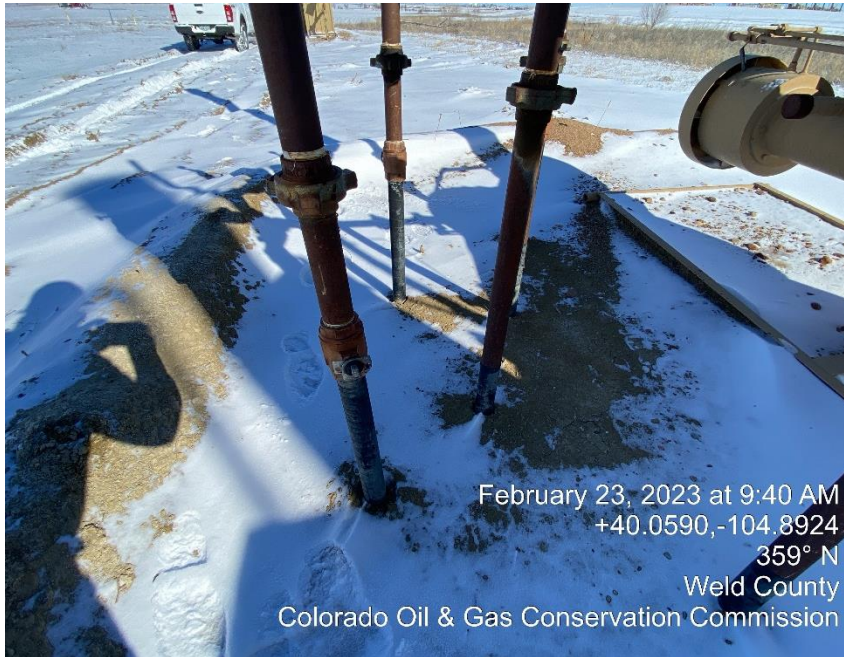
Photo #3 Balon valves appear to be open
