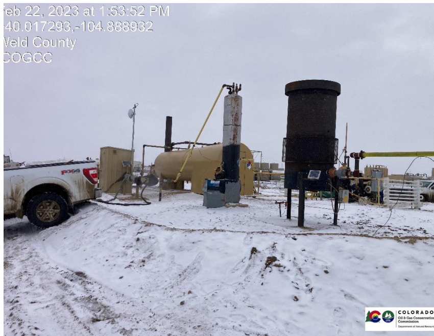
Pic 3. Spoke with KPK supervisor and was informed they were thawing lines on the gas meter run due to freezing issues, and changing oil in other equipment.
