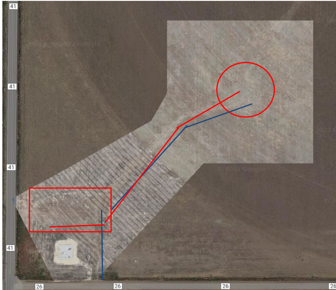
Photo 3. Orthomosaic drone aerial imagery taken from 200 ft (Oct. 2022). Illustrates rangeland growth on and around the well location (red circle), flowline (red line), tank battery (red rectangle) and access road (blue line). Tank battery area and access road still visible, so not full rangeland coverage.
