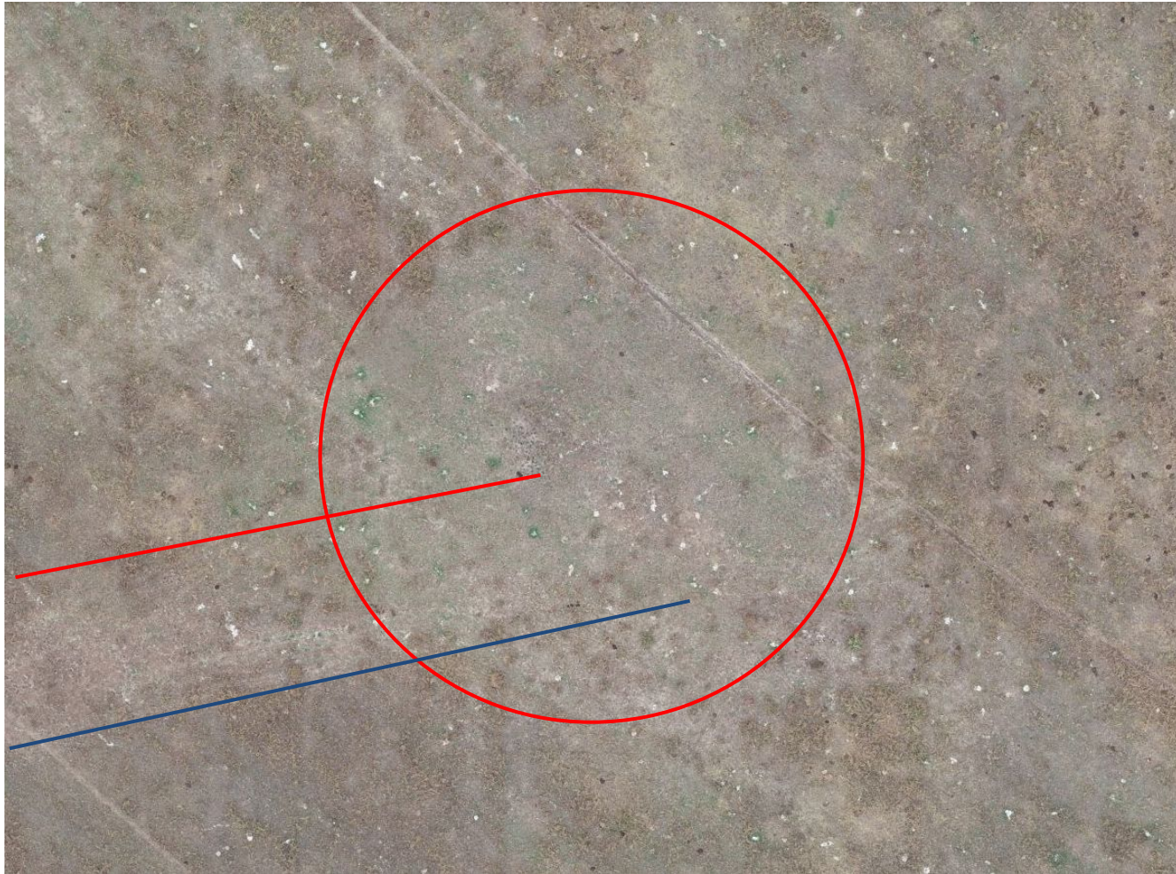
Photo 4. Zoomed in Orthomosaic taken from 200 ft (Oct. 2022). Illustrates rangeland growth on and around the well location (red circle) and access road (blue line). Comparable to surrounding area.
