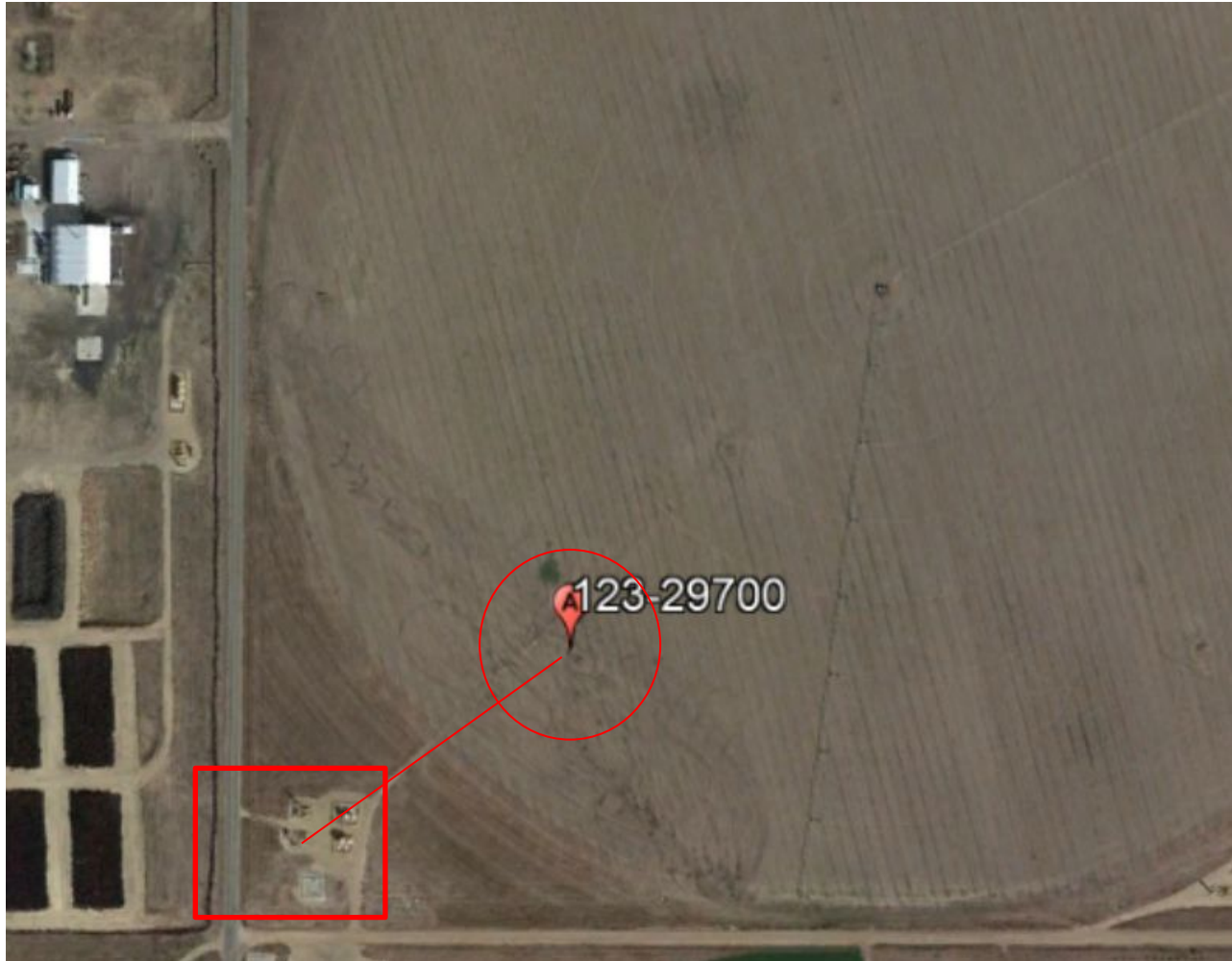
Photo 1. Google Earth aerial imagery taken 10/2015 during active operations. Photo illustrates the well location (red circle), tank battery (red square), and flowline (red line).
