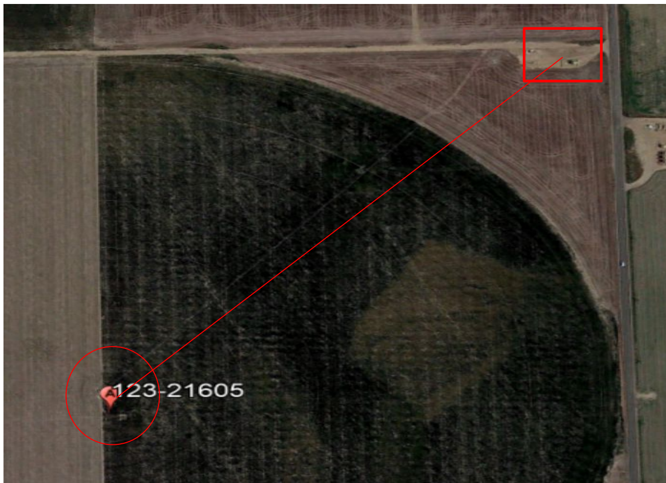
Photo 1. Google Earth aerial imagery taken 6/2017 during active operations. Photo illustrates the well location (red circle), tank battery (red rectangle) and approximate flowlines (red line).
