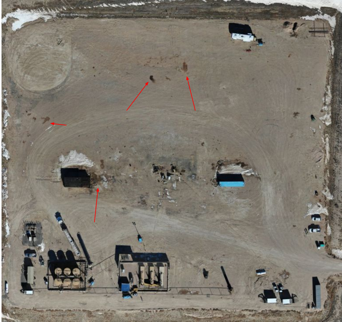
Photo 15. Drone aerial imagery illustrates stained soil throughout the location which has not been properly disposed of. Larger spills/releases were observed near frac tanks- refer to Photos 16-18. Red arrows indicate some of the stained soil and spills.
