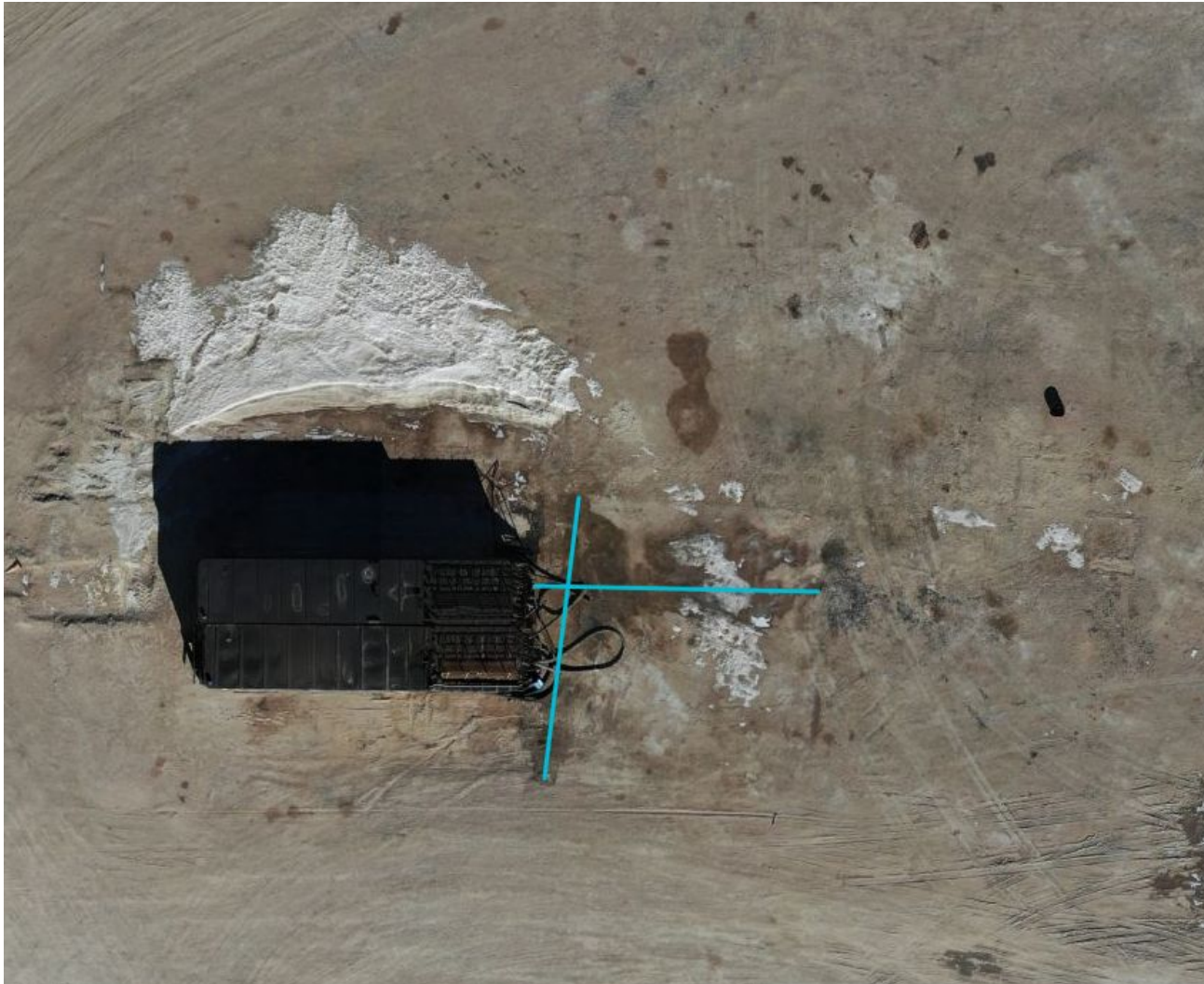
Photo 16. Zoomed in drone aerial imagery illustrates a larger spill/release near a frac tank. The blue lines indicate an approximate length of 37 feet. COGCC staff would consider this a reportable spill.
