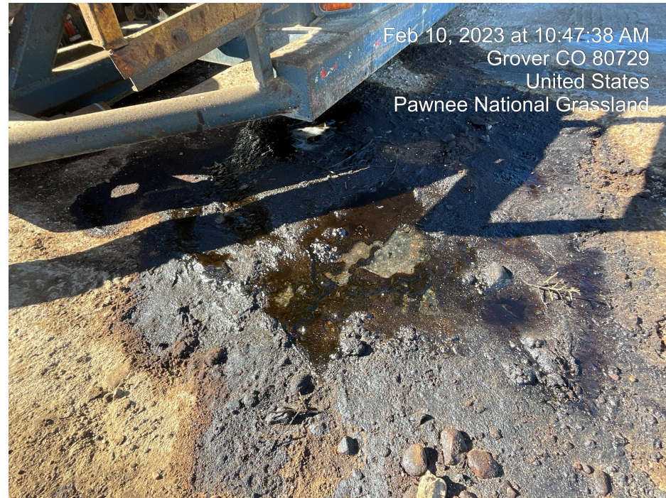
Photo 18. Close up photo of leaking frac tank from the previous photo.
