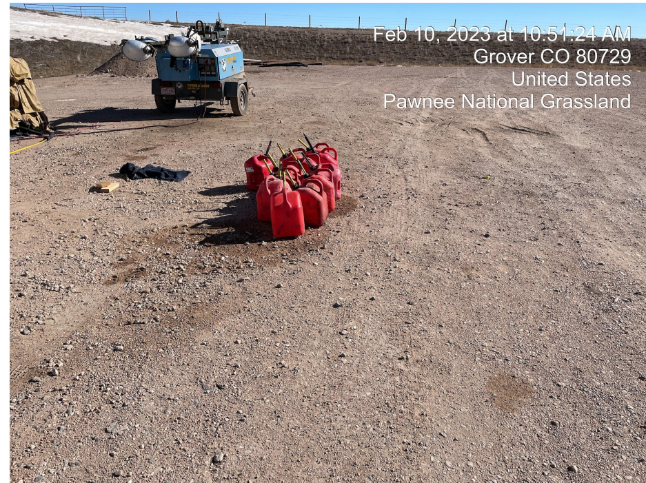
Photo 20. Photo taken from the northeastern location, facing East. Photo illustrates leaky gasoline. Operator does not have proper material handling and spill prevention.
