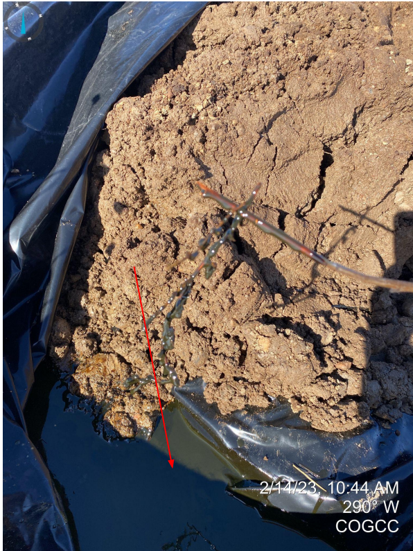
Photos 5 & 6. Close up photos illustrating pooling crude oil (left) and crude oil outside of the plastic liner.
