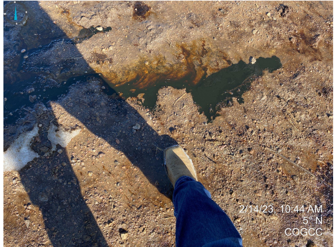
Photos 5 & 6. Close up photos illustrating pooling crude oil (left) and crude oil outside of the plastic liner.
