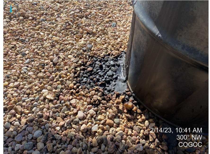
Photos 1 & 2. Facing northwest from inside of the tank battery containment. Photos illustrates an apparent leak originating from bucket/drum and staining the soil underneath.
