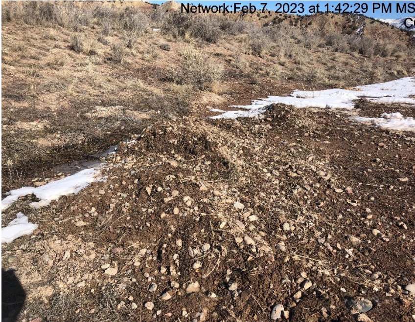
Photo #8936 Sediment has been transported into ditch.
