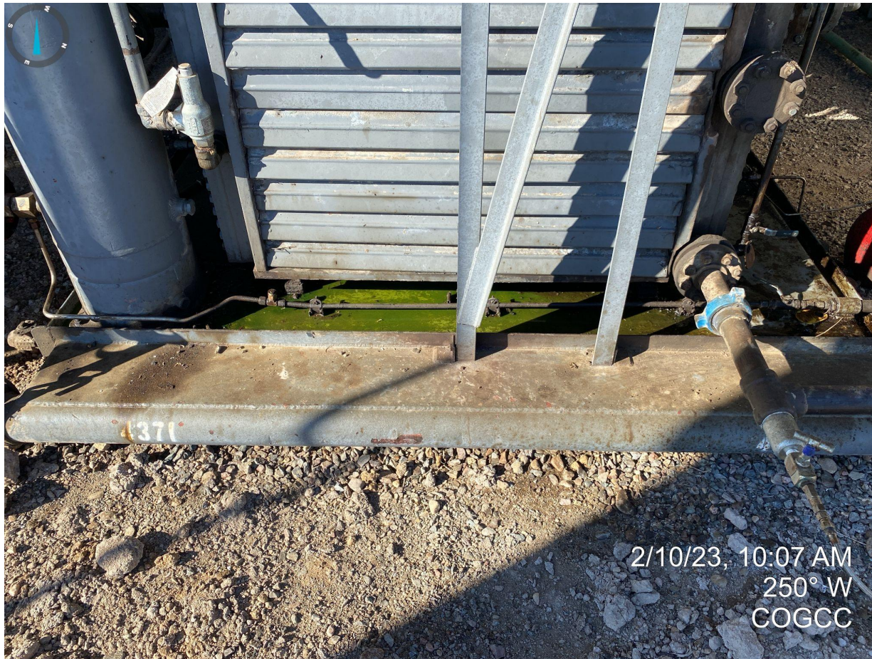
Photo 4. Close up photo of antifreeze spill observed on 02/10/2023.
