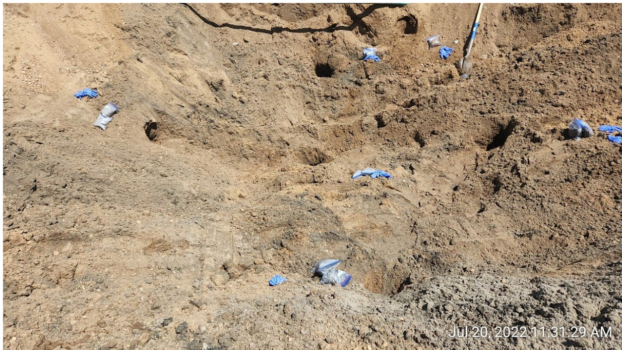
#2A – PTF-64N64W 32SENE – Base of Produced Water Vault Excavation – NPWVB01@5.0' – Staining and Odor Present – PID 1263ppm – Sample Submitted for Lab Analysis
