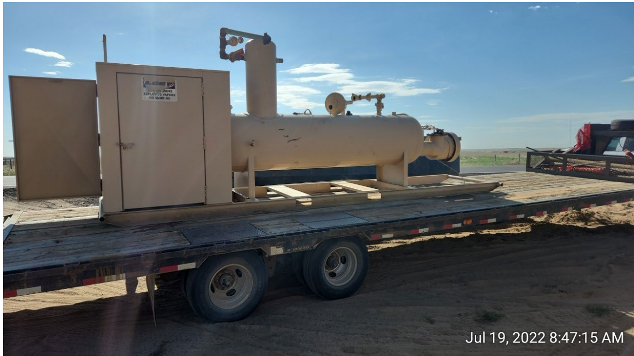
#4A – PTF-64N64W 32SENE – Separator – Good Condition – Minimal Corrosion
