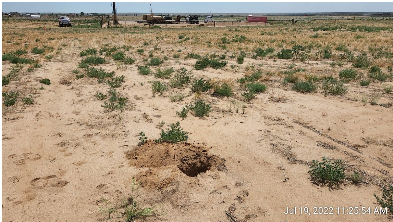
#7A – PTF-64N64W 32SENE – NBKG01@6.0" – No Impacts Noted – PID 0.1ppm – Sample Submitted for Lab Analysis
