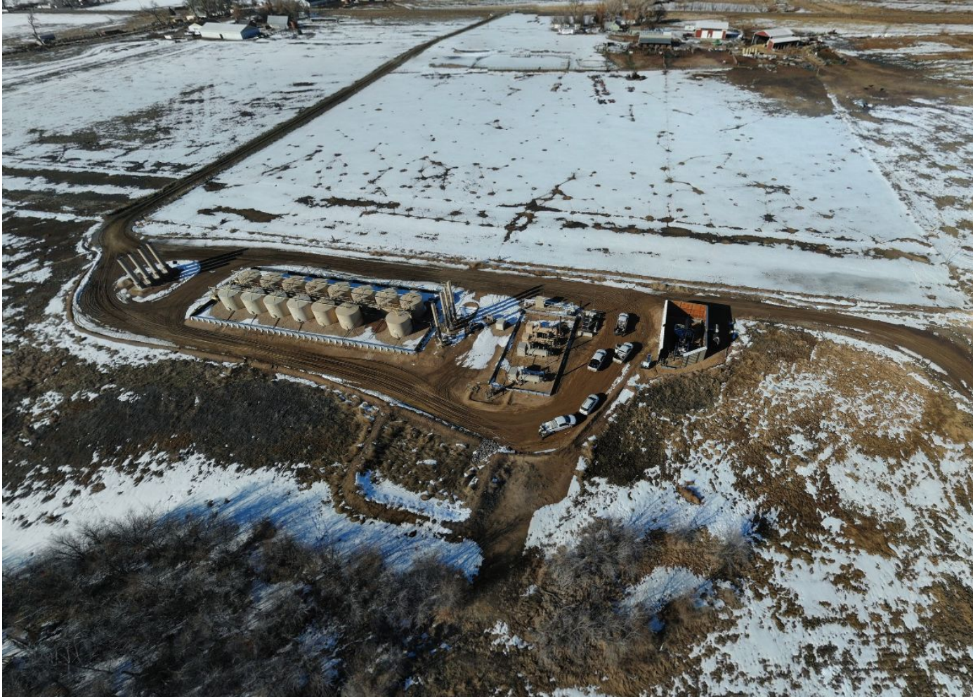
Photo 1. Drone aerial imagery from February 7, 2023 illustrates the Phelps facility and portions of the flowline area. COGCC observed stormwater while active snowmelt was occurring. Stormwater from the location is not being directed into the sediment trap and it appears only \frac{1}{3} of the facility might be directing stormwater to the sediment trap.
