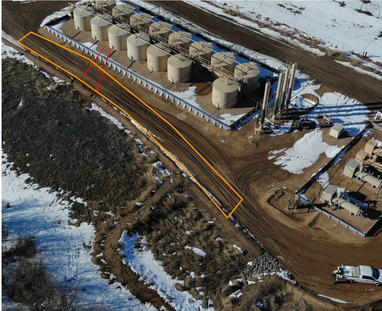
Photo 2. Drone aerial imagery from February 7, 2023 illustrates the earthen berm has failed and sediment laden stormwater is discharging off location. It appears that the other \frac{2}{3} of the location is pooling along the southern earthen berm which is not being directed into the inlet of the sediment trap.
