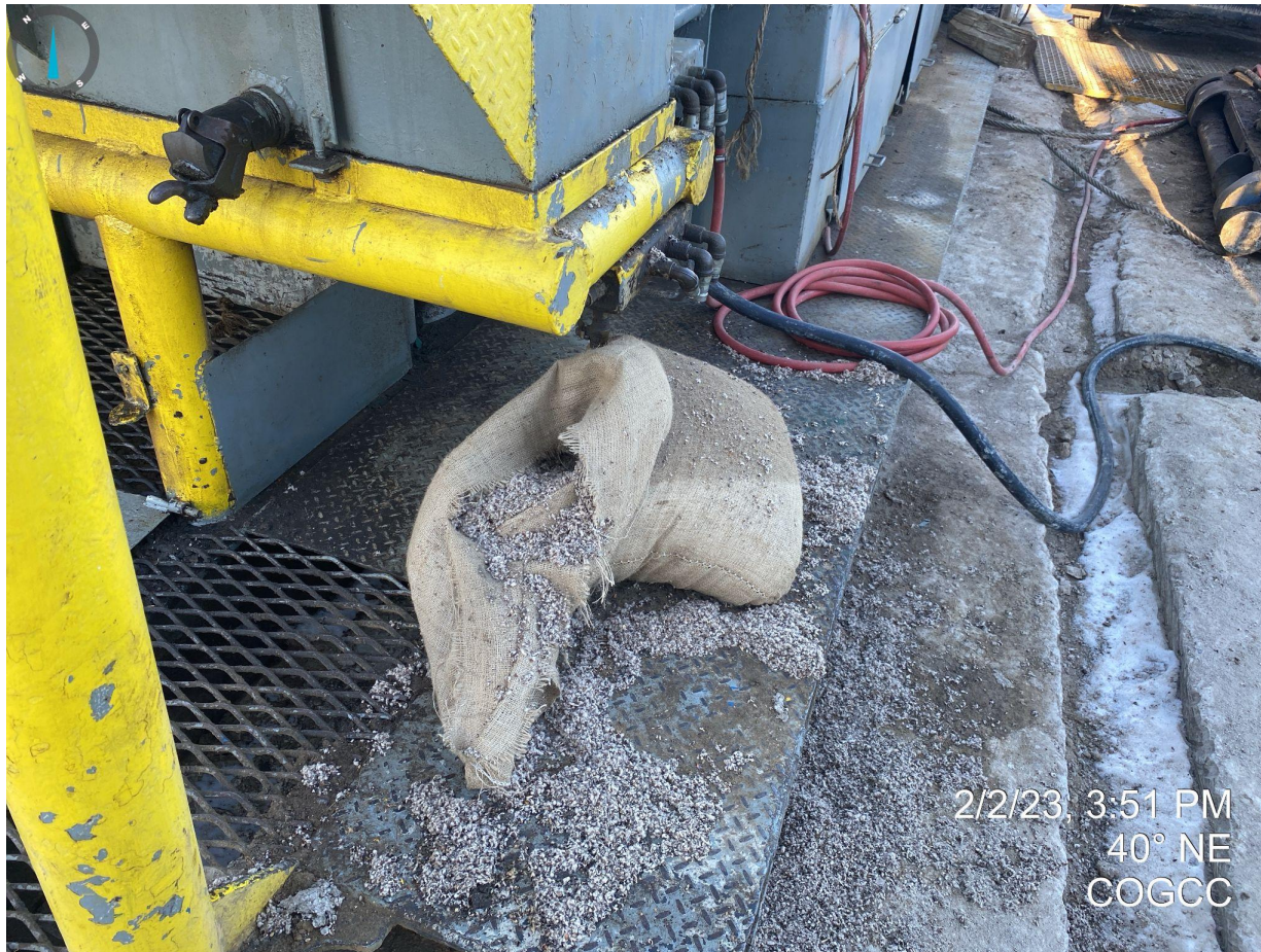
Photo 6. Facing northeast near drill rig. Photo illustrates that materials do not have adequate covering to minimize contact with precipitation or stormwater and are not in compliance with Rule 1002.f.(2)A.
