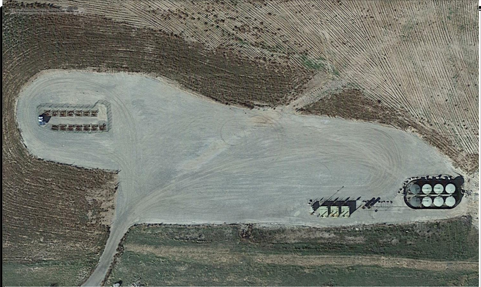
Photo 4: 2022 Google Earth Aerial image. Photos show areas of the current working pad between the wells, and the tank battery facility that are not reasonably needed for production operations, and require interim reclamation.
