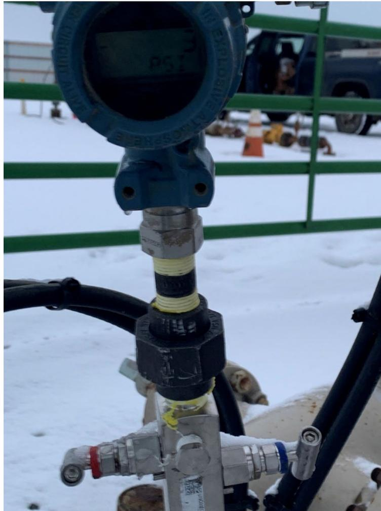
**CA:** Rush 3AH bradenhead 0 psi, Little Rush bradenhead is not connected. Inspector could not check the bradenheads on the 4 new wells bc the rig was on the 005-07455 well. Install appropriate fittings to allow bradenhead visual inspection as per Rule 419.a.(1), (2).
