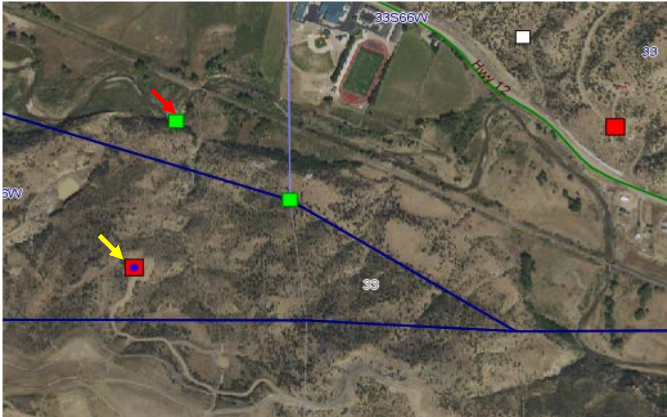
Photo 1. The associated pit has incorrect coordinates showing the pit at red arrow and the well site is shown at yellow arrow.
