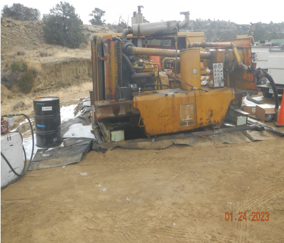
Photo 3. There are multiple equipment leaking oil. There is plastic matting however it does not cover the area well and has no containment.
