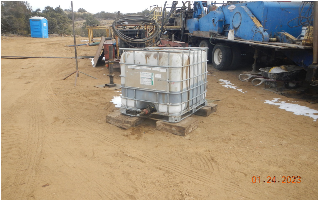
Photo 20. There is stained soils at the outlet of this oil container which is not properly stored.
