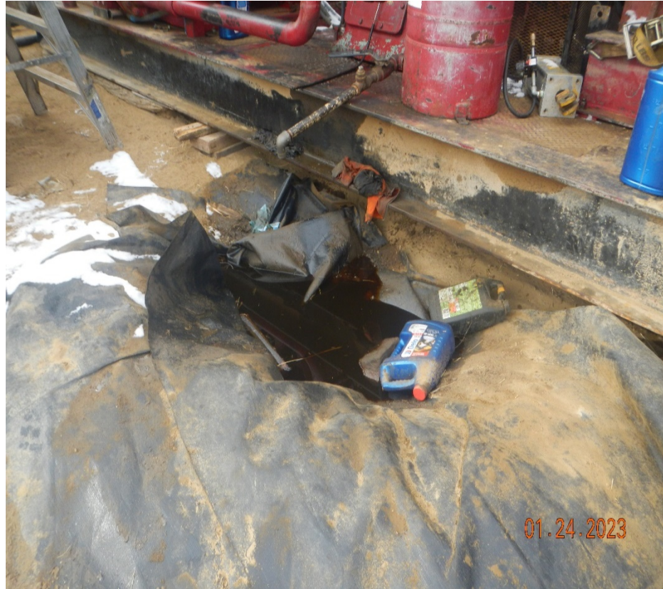
Photo 8. There is oil leaking out of this engine skid which is not contained and containers laying on the ground.
