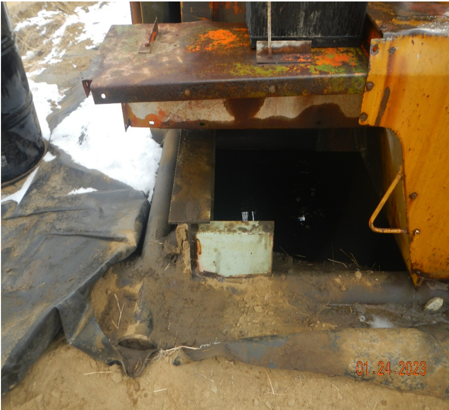
Photo 5. There is oily fluid in tis engine skid which is not contained and needs to be cleaned up immediately.
