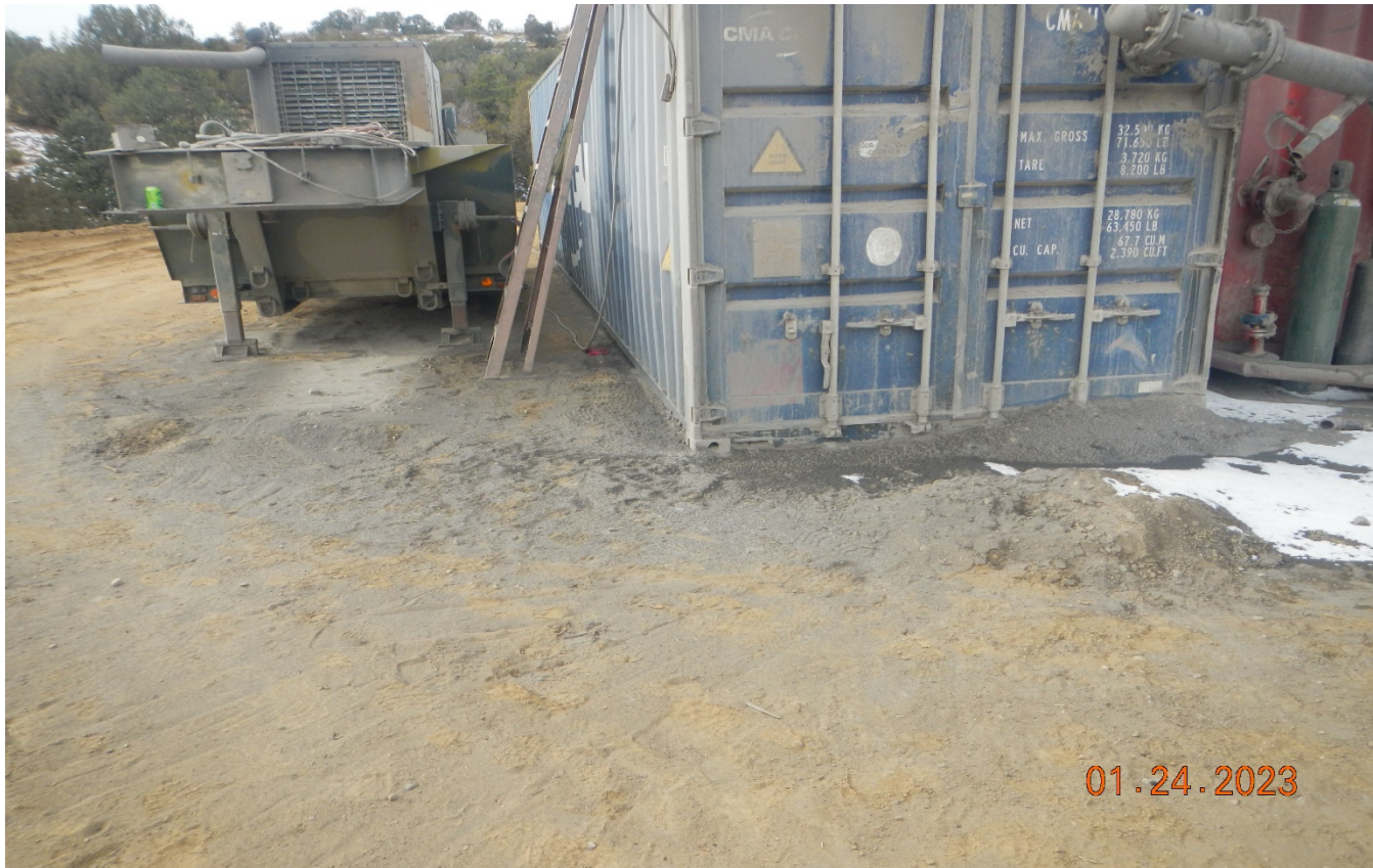
Photo 19. There is drill cuttings on the surface not properly stored and contained.
