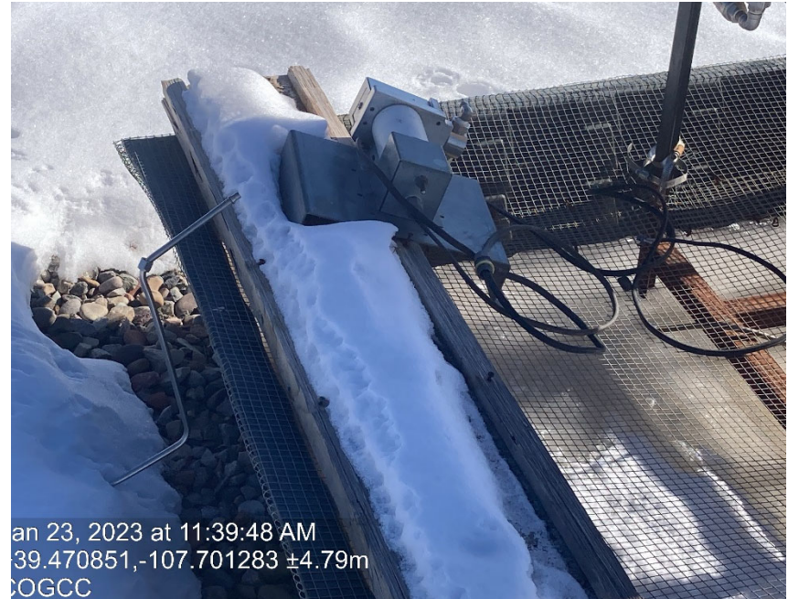
Unused chemical tank (disconnected and missing equipment for pump to operate)
