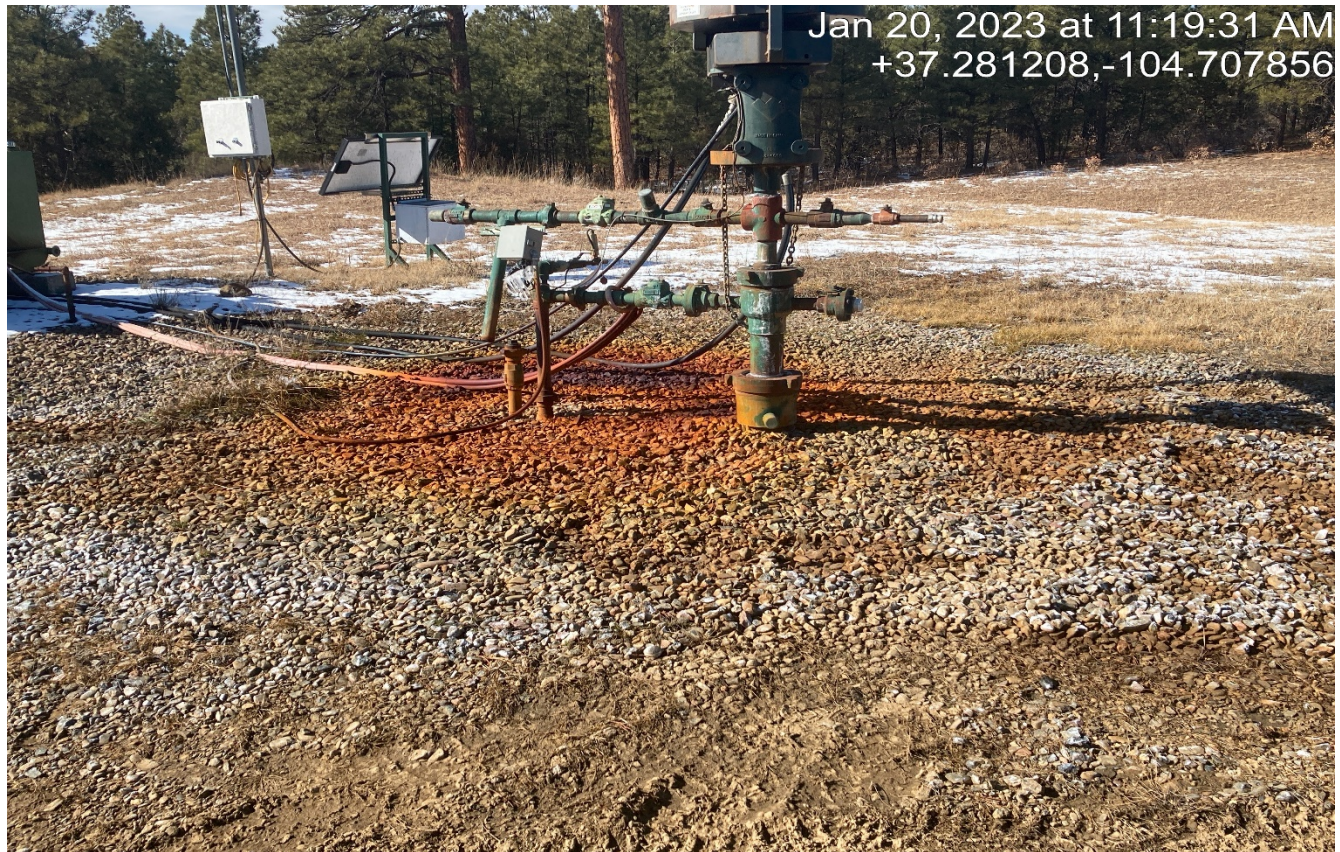
Photo 3. There is stained soils at the wellhead that needs to be cleaned up.
