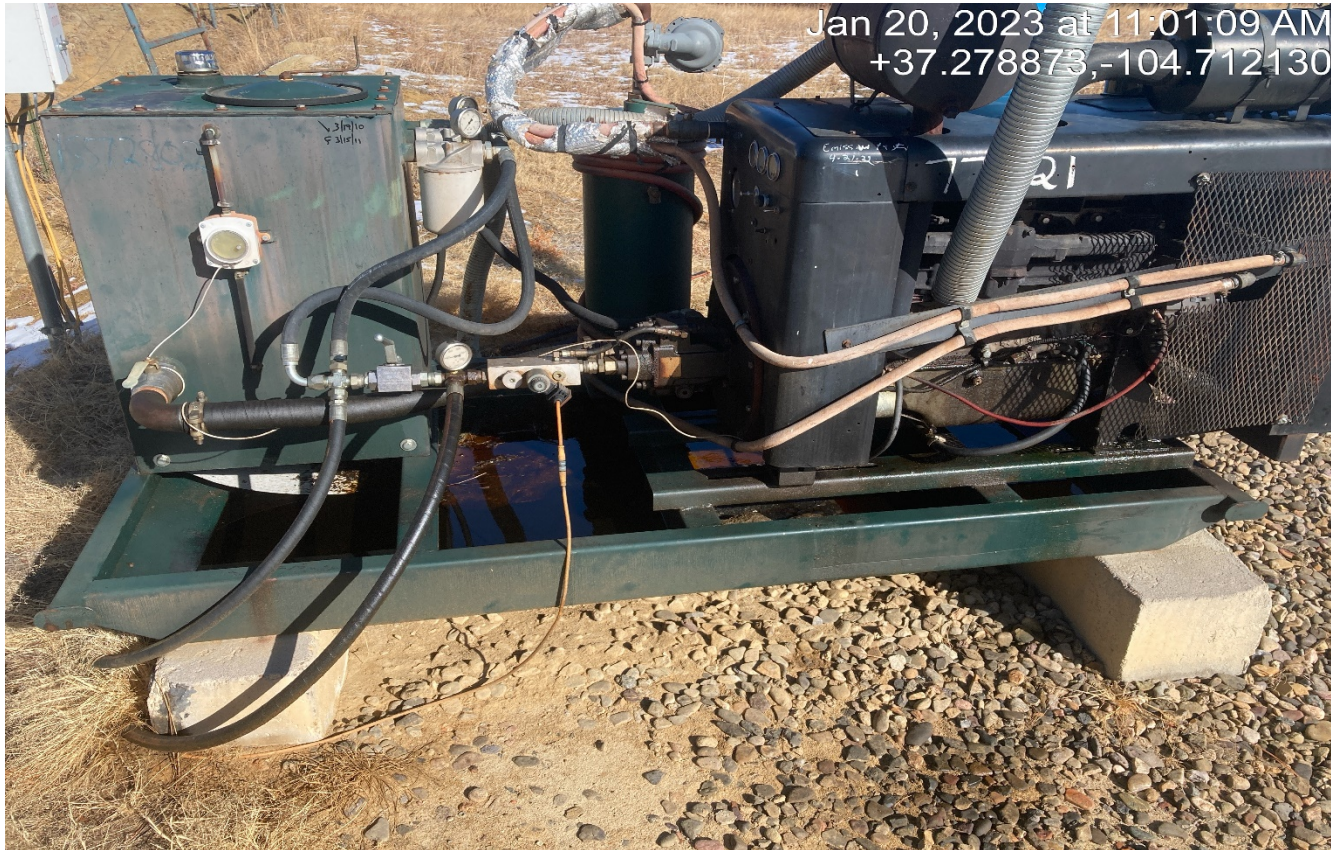
Photo 3. There is some oily waste in the engine skid that should be cleaned up.
