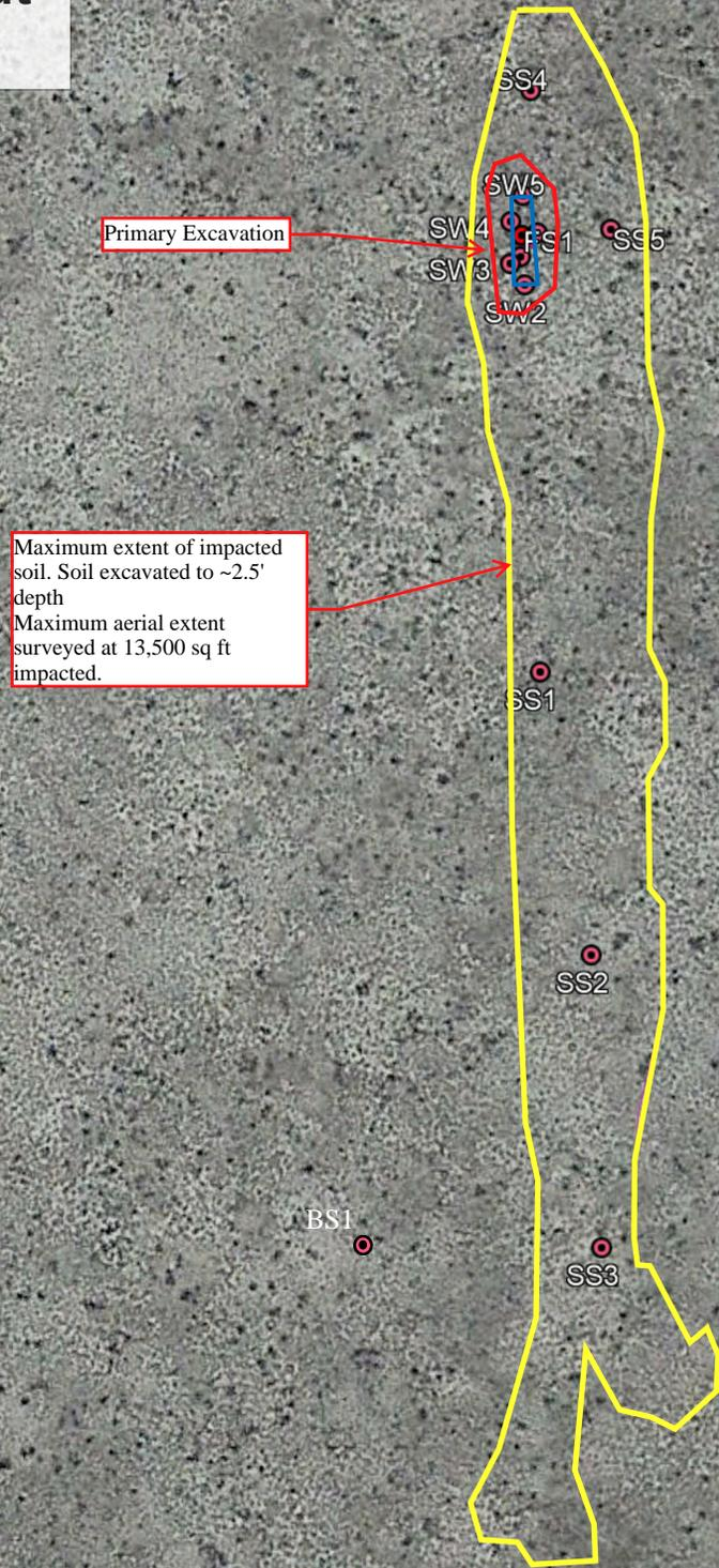
Maximum extent of impacted soil. Soil excavated to ~2.5' depth
