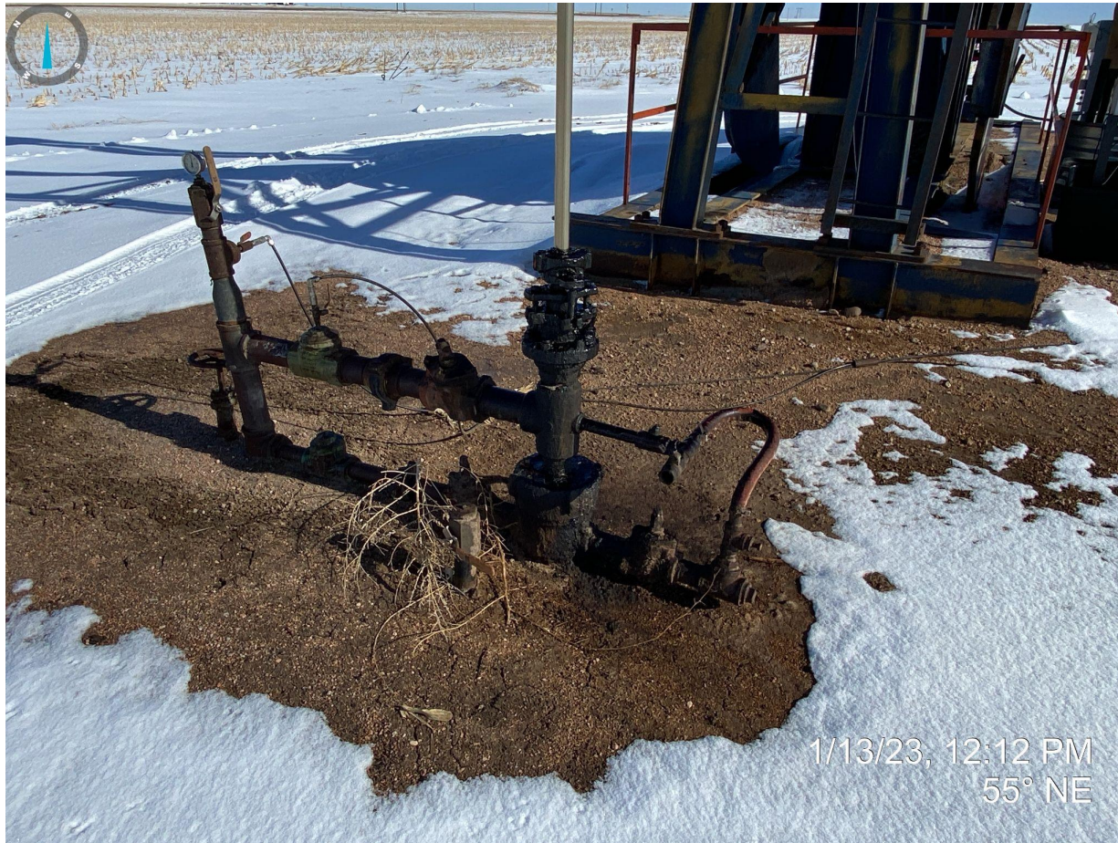
Photo 8. Facing northeast from wellhead. Photo illustrates oil stained soil around wellhead that needs to be properly cleaned and disposed of.
