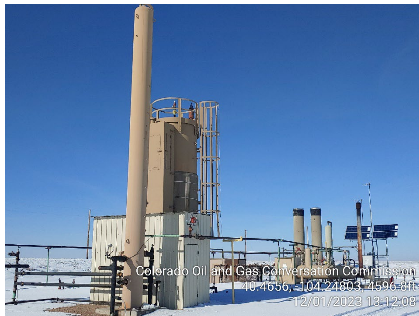
Photo 6 – VRT and Heater Treater
