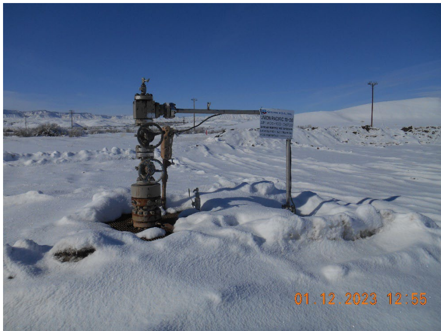
Injection wellhead
