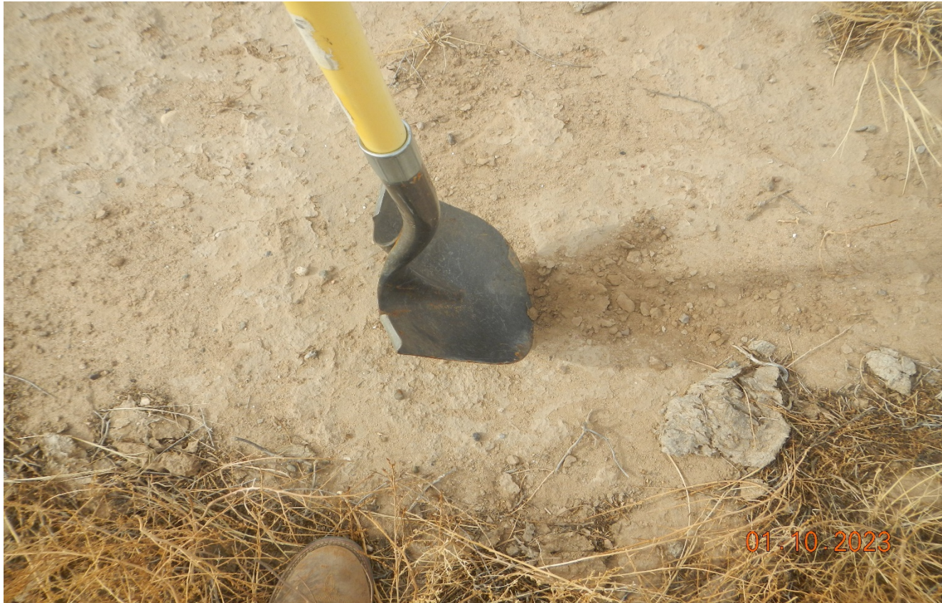
Photo 4. The soils were not decompacted. The shovel shown in the photo could not penetrate the soil surface.
