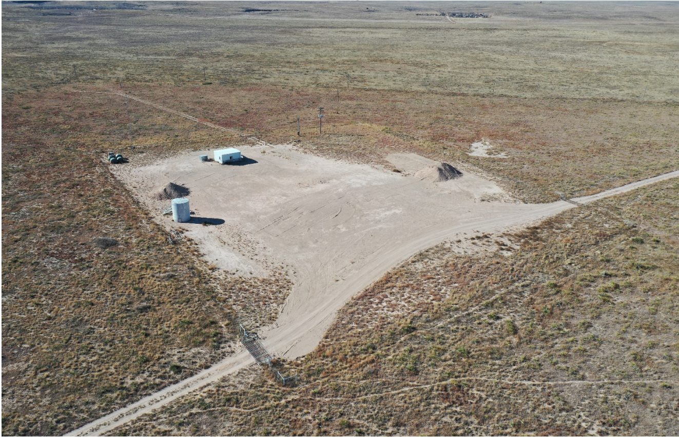
Photo 7. Drone aerial photo facing west toward the TANNER SEC REC UNIT #501 well site and production facility. The abandoned facility and well site has not been reclaimed and equipment remains. This image was taken during previous inspection.
