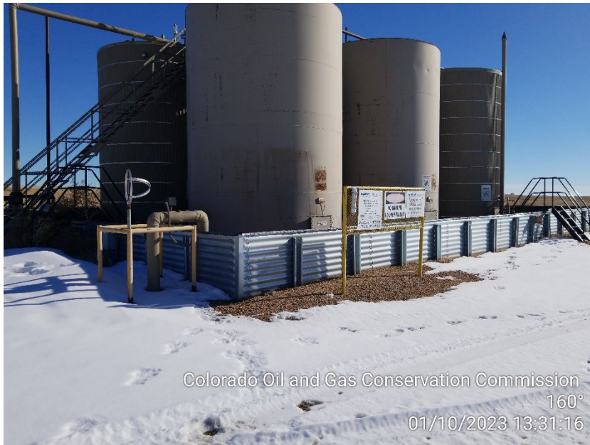
Photo 7 – Tank Battery
