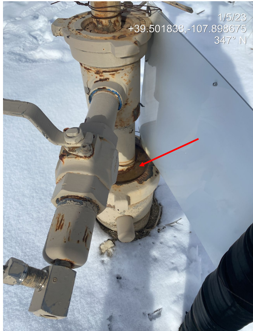
Photo 2. Photo shows where bubbles were observed to be rising in water around the wellhead.
