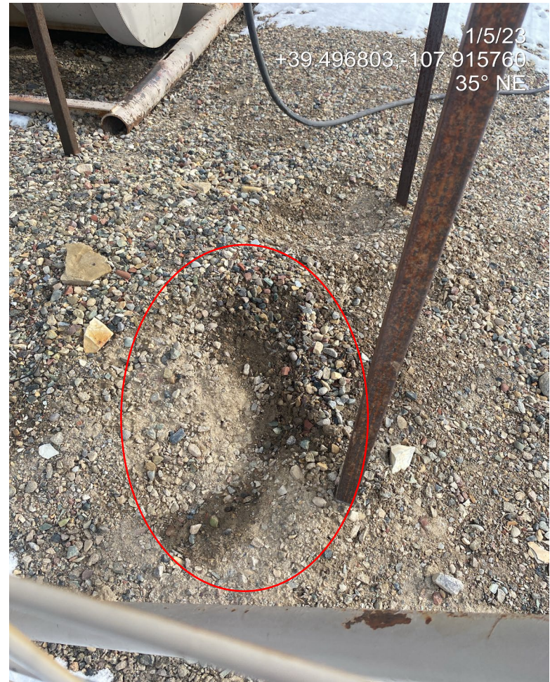
Photo 2. Photos show stained soil beneath chemical injection equipment at the separators.
