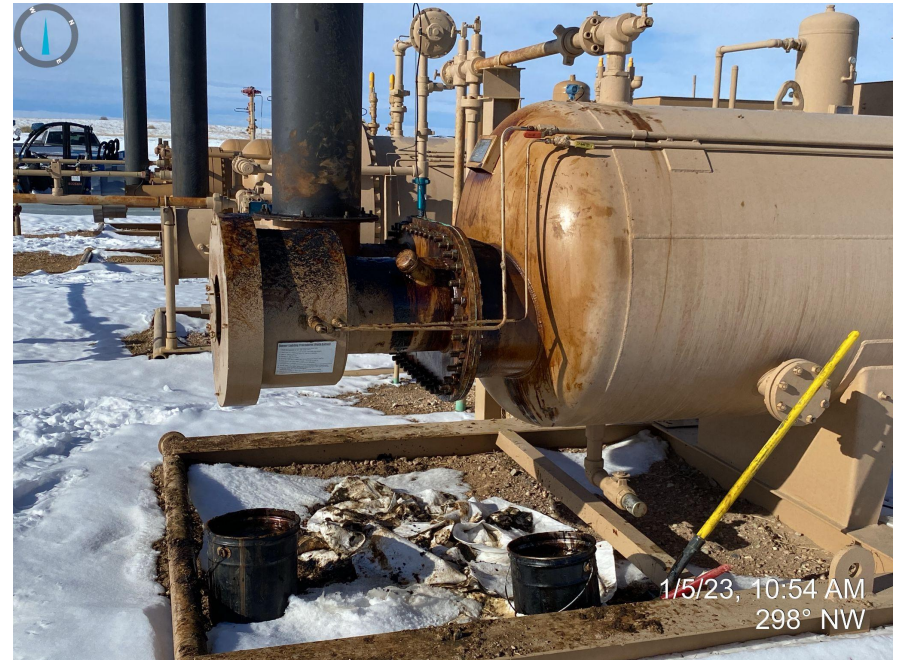
Photo 4. Facing northeast/northwest towards separator at the north end of the location. Photos illustrates a failed gasket that resulted in fluid exiting the equipment.
