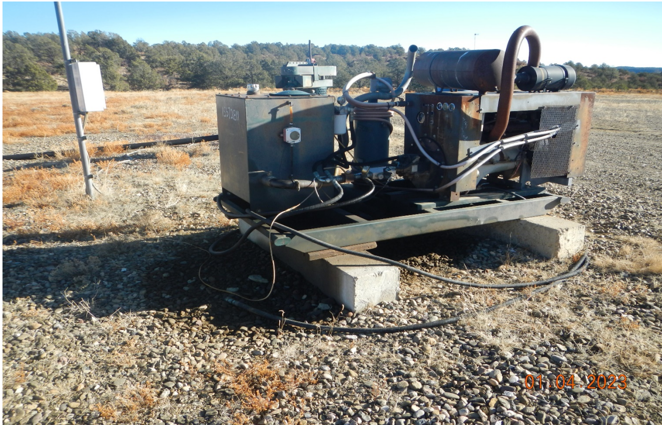
Photo 2. There are oil stained soils at the engine skid that needs to be cleaned up.
